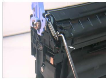
10. Release the spring on the gearless side.
