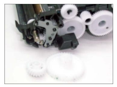
**REMOVING THE DEVELOPER GEAR SUPPORT PLATE** 18. Remove the developer drive gears shown.
