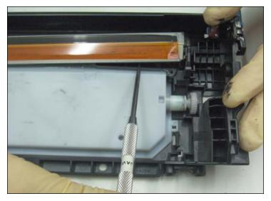
40. Wedge a small scriber or small screwdriver between the base of the wiper blade and the hopper beneath that it adheres to.
