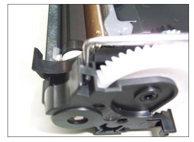
14. Locate the first tab on top of the end plate. Using a hook tool, push the tab away to release.
