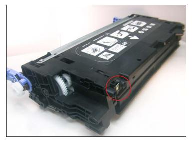
**CHIP REPLACEMENT PROCEDURE** 43. Locate the OEM chip near the top rear of the remanufactured cartridge
