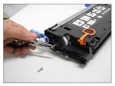
7. Go to the opposite Gear side and repeat the extraction procedure. This pin also passes thru the center of the main drive gear during extraction.
