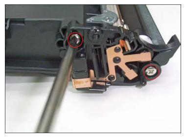
**REMOVING THE GEARLESS SUPPORT PLATE** 23. On the opposite end of the hopper, remove the two screws shown that hold the developer roller gearless support plate in place.
