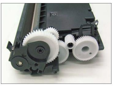
**REMOVING THE DEVELOPER ROLLER END PLATE** 13. We will begin with the removal of the end plate on the gear-side. The end plate is held in place by three interlocking tabs.
