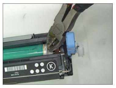
31. Rotate the OPC so the pin is visible and able to grasp using medium-sized pliers. Extract the pin by pulling it out.
