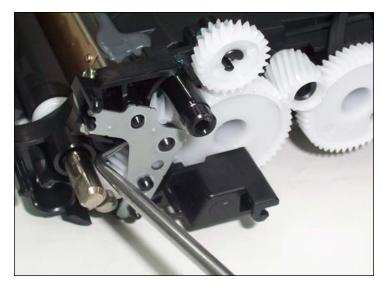
19. Using a hook tool, slide out the gear retaining plate. This will reveal three remaining drive gears beneath.
