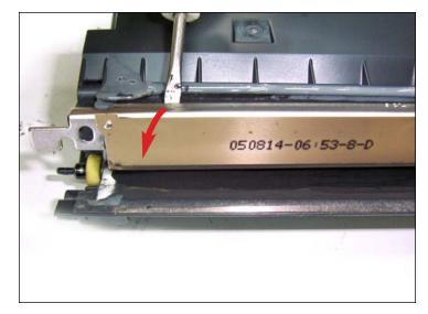
27. Using a small flathead screwdriver, pry the blade far enough to separate it from OEM adhesive.
