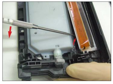
41. Position the scriber over the waste hopper shown for support as you push downward, prying the wiper blade assembly up and releasing it from its adhesive seal.
