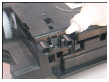
48. Apply a small amount of plastic cement into the plastic slots. This will seal the replacement chip into place from each side.
