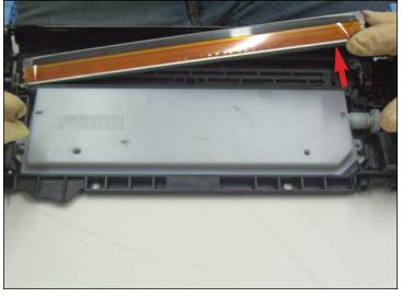
42. Now slowly but firmly, pull the loose end of the wiper blade upward with your hand as shown until is completely removed.
