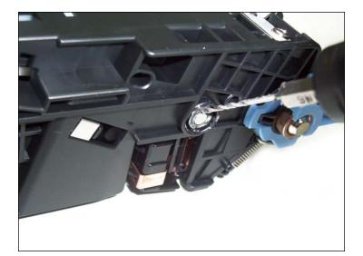
3. Drill a small hole just above the pin on both sides of the cartridge.
