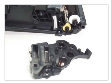
24. Slide off the gearless support plate.
