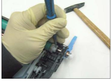
**DISASSEMBLING THE DRUM UNIT** 30. Using a chisel and hammer, hammer out the locking pin through the other side of the drum using swift hard blows.
