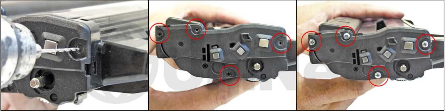
33 Drill four small holes that correspond to the screw size your using.
