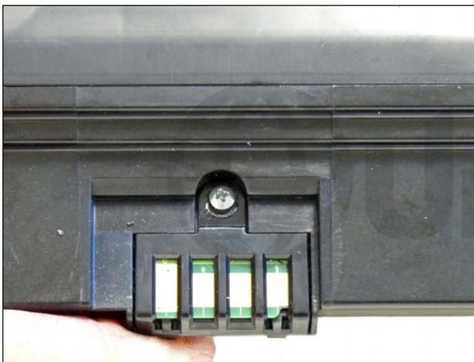
39. Install the new chip and cover, and insert a small screw that corresponds to the hole drilled to hold everything in place. It's very easy when drilling the hole for this screw to drill through into the waste chamber. Place a small amount of silicone caulk in the hole and screw before install the screw.
