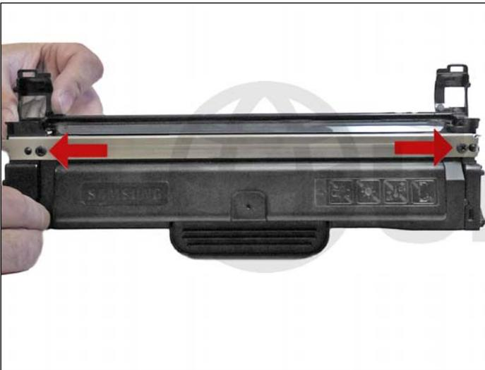
23. Remove the two screws from the doctor blade, and remove the blade. Clean out all the remaining toner from the hopper.
