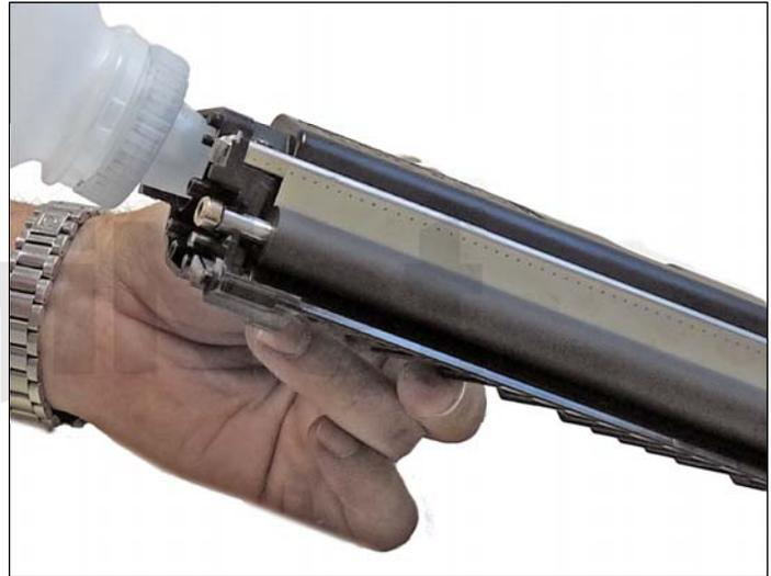
28. Fill the hopper with toner for use in Dell 1130, replace the fill plug, and check for leaks.
