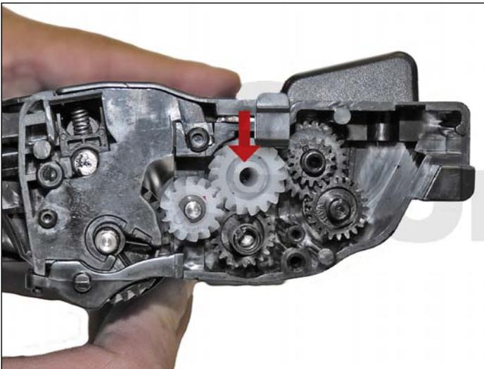
34. Install the large white floating gear on the gear side of the cartridge.
