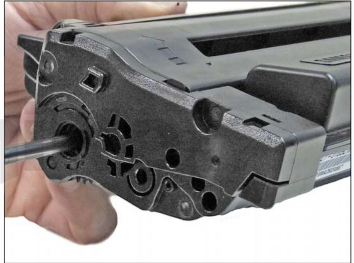
3. Remove the drum axle arm from the right or large gear side of the cartridge.
