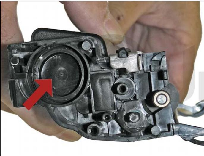
21. On the supply hopper, carefully pry out the fill plug and dump out any remaining toner. The fill plug can be difficult to remove as it is recessed. Take a small common screwdriver and work it around the edge lifting slightly until it comes loose.
