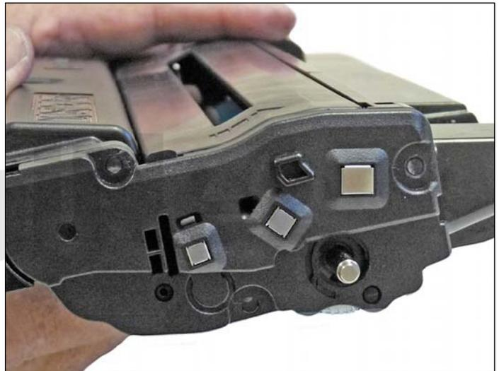
32. Clean the contacts on the left side end cap, and replace the conductive grease.
