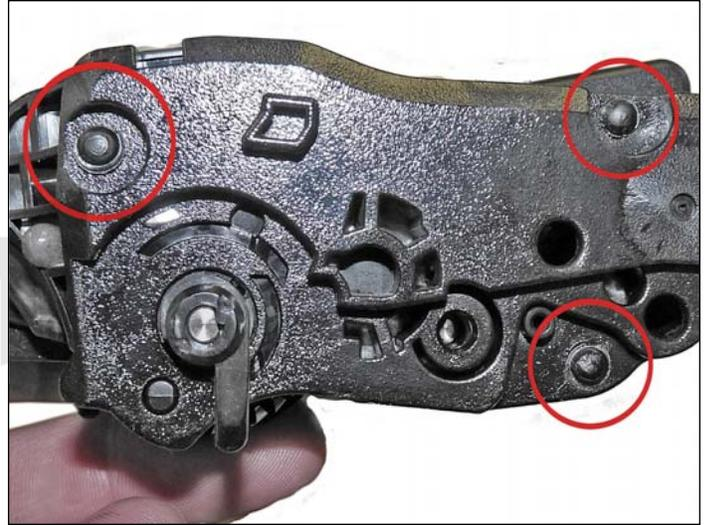
These cartridges have taken a dramatic change in that there are no screws in the outside of the cartridge at all. There are plastic rivets that need to be cut off, holes drilled and screws installed to hold them back on. It's not a hard process and it's covered completely in the instructions.
