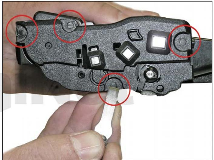
2. On the right side end cap take the chisel blade knife and slice off the heads of the four plastic rivets.
