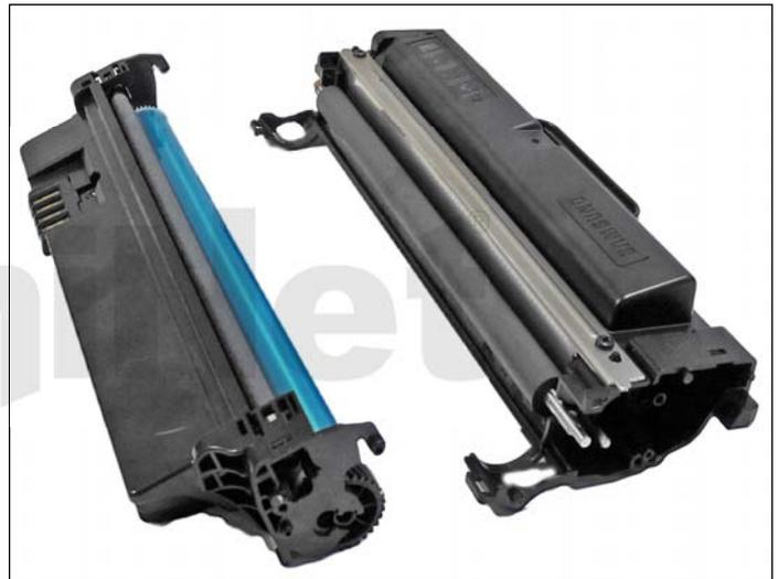
8. Lift up on the drum/waste hopper and remove.
