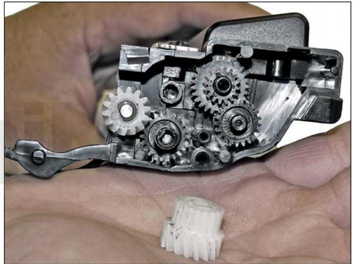
29. Install the gears as shown.
