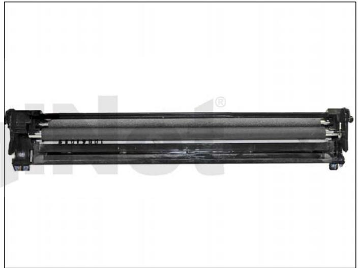
18. Place a small amount of conductive grease in the holders,
