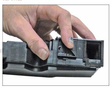
3. Remove the waste chamber. Slide the cover open and vacuum/blow the waste chamber clean.
