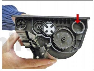
6. Remove the toner fill plug. Dump the bulk of the remaining toner out of the cartridge. Vacuum/blow out the toner supply chamber clean. It is not necessary to get the cartridge completely clean now, as the developer roller needs to come out so the doctor blade can be cleaned. You will have easy access to clean out the hopper then.
