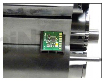
15. Replace the chip on the cartridge. Note that the OEM chip is an RF type chip built on a flexible label.
