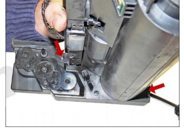
9. Install the waste chamber and three screws.
