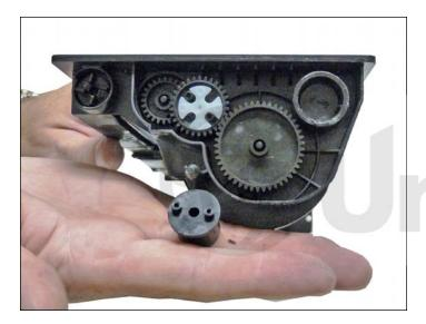
5. Remove the large drive gear.
