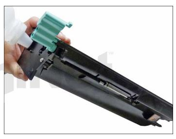
13. Fill the cartridge with 4150 toner. Replace the fill plug.
