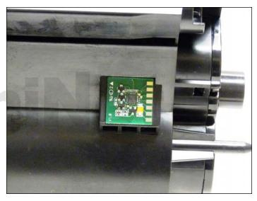
10. Replace the chip on the cartridge. Note that the OEM chip is an RF type chip built on a flexible label.
