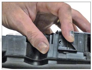
11. Remove the waste chamber. There are two small gears that will come loose.
