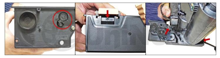
14. Install the two gears on the hopper. Install the waste chamber and three screws.
