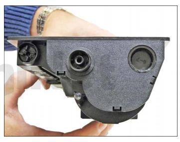
8. Angle the top tabs in first and snap the cover back in place.
