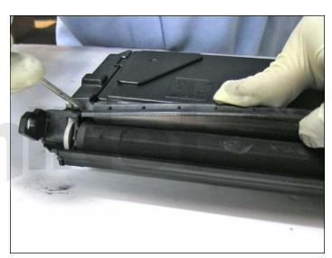
4. Using a flathead screwdriver, pry loose the doctor blade cover from either side of the toner cartridge as shown.
