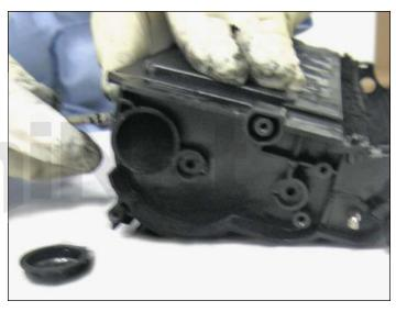
18. Using a pair of needle-nose pliers, pull out the toner fill cap found on the gearless side of the cartridge. You are now ready to empty and clean the toner cartridge.
