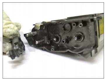
16. Gearside developer roller support removed.
