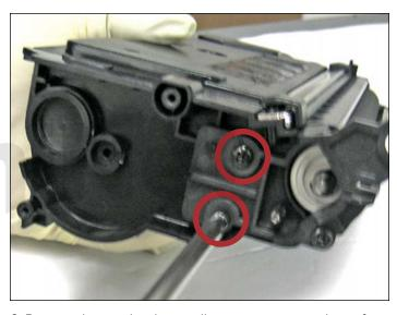
6. Remove the two developer roller support screws shown from the gearless side of the cartridge.
