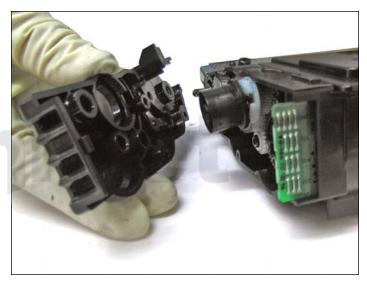
10. Remove the gearside end cap.
