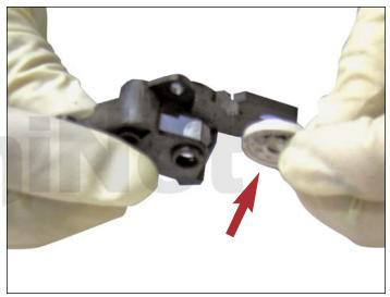
8. Gearless side developer roller support shown with bearing attached.
