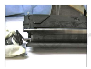
7. Gearless side developer roller support removed.
