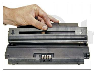
34. Install the cleaned PCR cleaning roller cover assembly.
