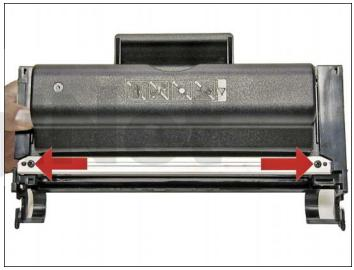
14. Remove the two screws on the doctor blade.
