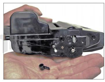
2. Gently pry off plastic drum axle bushing. Keep this bushing with the appropriate end cap when removed. Each side is different.
