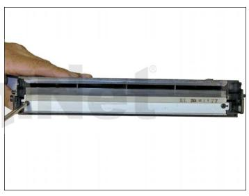
27. It is interesting to note that on new cartridges, some toner is in the waste hopper. Apparently these cartridges are being tested before they are shipped, or the drum was lubricated with toner.
