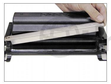
15. Carefully pry up the doctor blade. This blade has a very tight fit, so work it off carefully. Clean out any remaining toner from the hopper.
