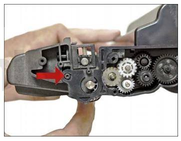
8. Carefully pry up the side plastic tab to release the waste chamber.
