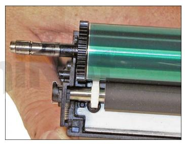
31. Install the drum axle, small drum gear side first.
