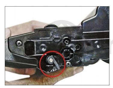
38. Press the drum axle bushing in place. Set it so the small tab is at the end of the groove; make sure it is fully seated. The two small bushings are different. Make sure you have the correct bushing for this side.
