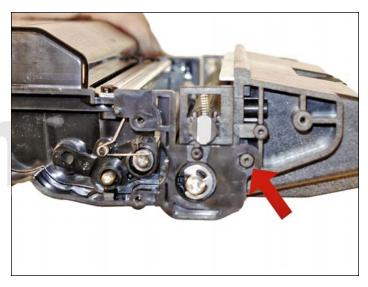
33. Install the waste hopper on to the supply chamber.
