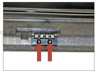
39. The chip is held in place by plastic rivets. It must be replaced for the cartridge to work. It can be replaced by cutting the plastic rivets, drilling two holes, and setting two self-tapping screws in place.
