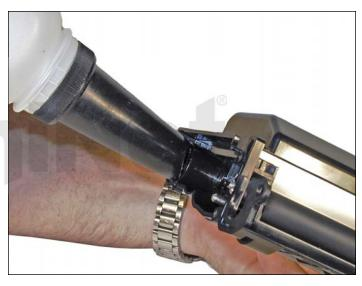
21. Fill the hopper with 135g or 290g of toner for use in Xerox WorkCentre 3550. Check for leaks.
