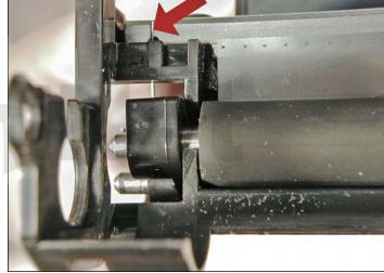
19. Snap the spring/plastic bushing assembly in place.
