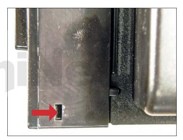
37. Remove the tape from the gears, and install the left side end cap and three screws.
