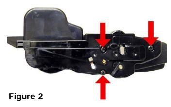
2) Gently pry off plastic drum axle bushing. Keep this bushing with the appropriate end cap when removed. Each side is different. See **Figure 3**
