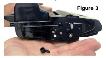
3) On the top edge of the end cap, there is a plastic tab. Press in on the tab and remove the right end cap. See **Figures 4 & 5**
