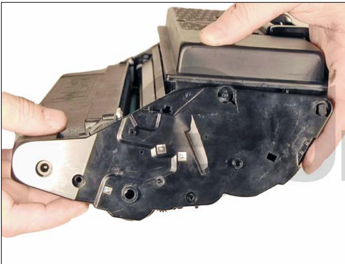
58. Pull the seal tab through the end cap seal slot.
