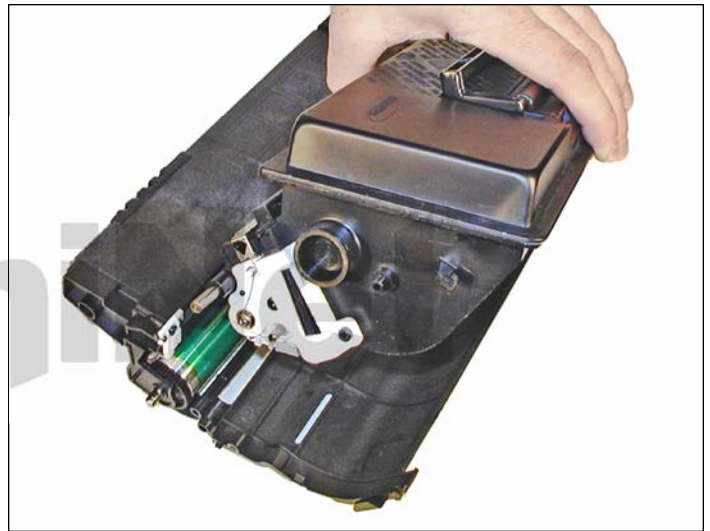
10. Remove the toner hopper from the frame.
