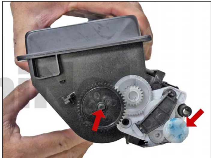
47. Install the large black gear and the small white drive gear.
