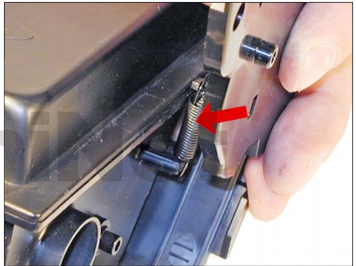
57. Install the spring from the end cap to the hopper.
