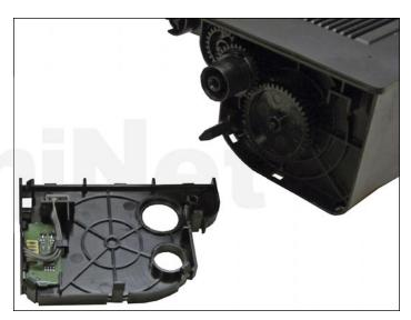
9. Press in on the four tabs on the opposite side of the cartridge.
