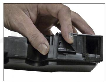
3. Remove the waste chamber. There are two small gears that will come loose.
