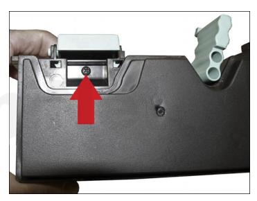
2. Remove the screw that is located under the colored plastic handle.
