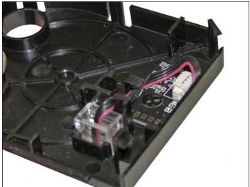
10. Replace the chip on the cartridge.
