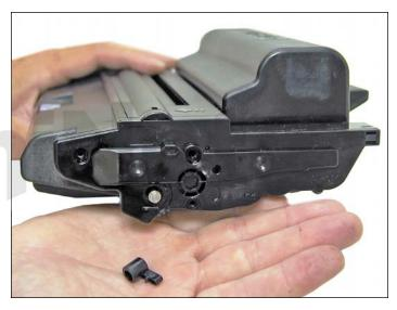
5. Gently pry off plastic drum axle bushing. Keep this bushing with the appropriate end cap when removed.
