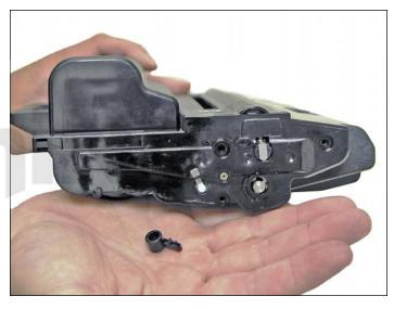
2. Gently pry off the plastic drum axle bushing. Keep this bushing with the appropriate end cap when removed. Each side is different.
