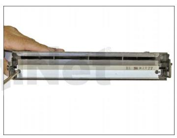
27. Coat the new wiper blade with your preferred lubricant. Install the new wiper blade and two screws. The tail of the wiper blade should face up.
