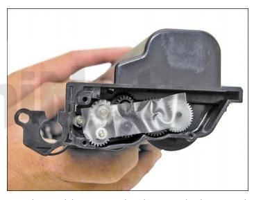
11. Remove the developer roller drive gear; place a strip of tape across the remaining gears as they do not need to be removed.
