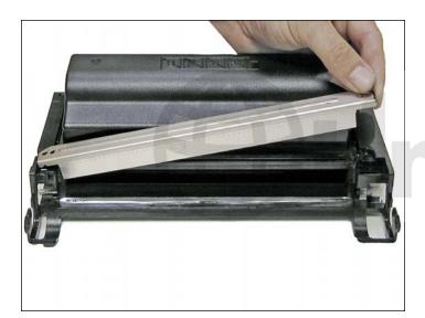
15. Carefully pry up the doctor blade. This blade has a very tight fit, work it off carefully. Clean out any remaining toner from the hopper.
