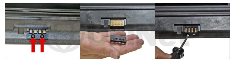
39. The chip is held in place by plastic rivets. It must be replaced for the cartridge to work.
