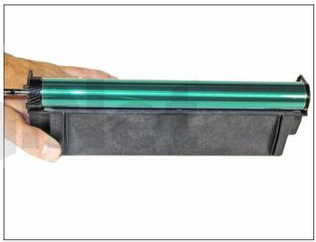
23. Slide the drum axle out from the side opposite the E-ring (large gear side).
