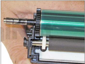
31. Install the drum axle small drum gear side first.
