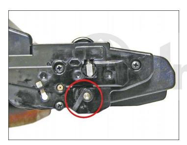
36. Press the drum axle bushing in place. Set it so the small tab is at the end of the groove; make sure it is fully seated. The two small bushings are different. Make sure you have the correct bushing for this side.
