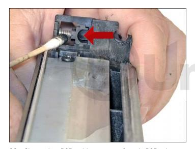
28. Clean the PCR with your preferred PCR cleaner. **WARNING**: Do not clean the OEM PCR with alcohol, as this will remove the conductive coating from the roller. If the PCR is an aftermarket, follow the cleaning methods recommended by the manufacturer. If the PCR is an OEM, we recommend it be cleaned with your standard PCR cleaner.
