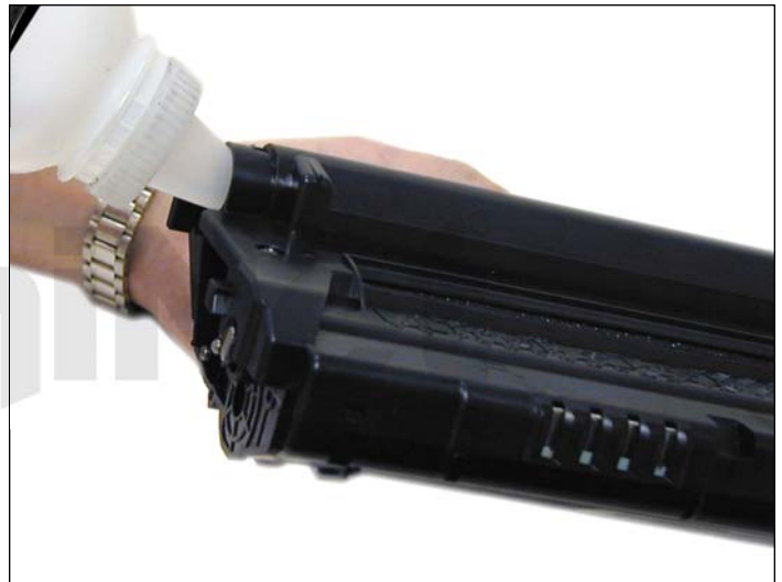
23. Fill the hopper with toner for SCX-4300.
