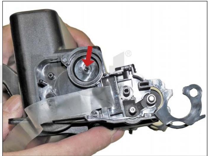
34. Fill the hopper with toner for use in Samsung ML-3712.
