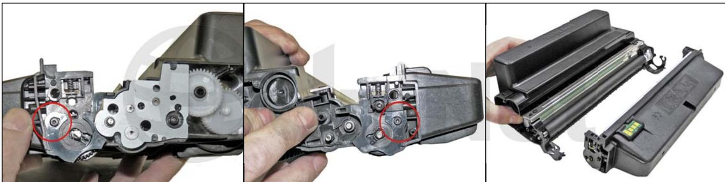
8. Gently pry up on the tabs on both sides of the cartridge and remove the waste hopper.
