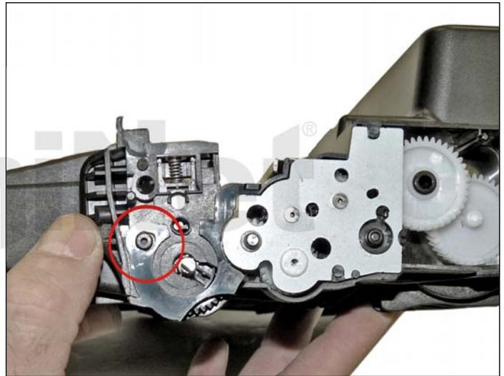
38. Fit both sides of the waste hopper tabs into the toner hopper.
