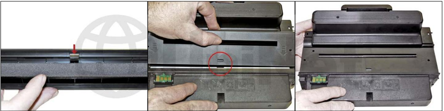
39. Slide the cleaned middle top cover/PCR cleaner assembly into place.
