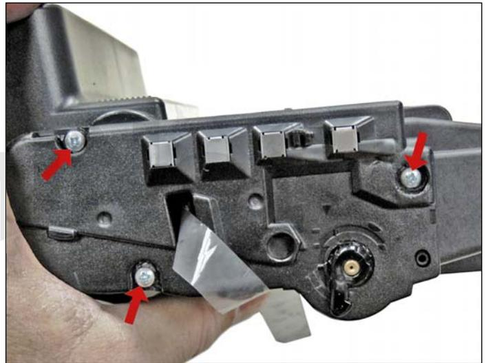
41. Drill three small holes that correspond to the screw size you're using.
