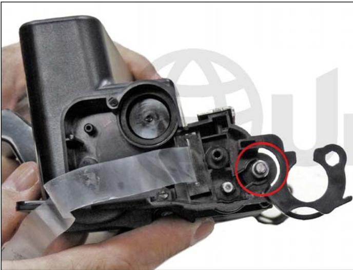
33. Clean and replace the conductive grease on the short shaft side of the roller.
