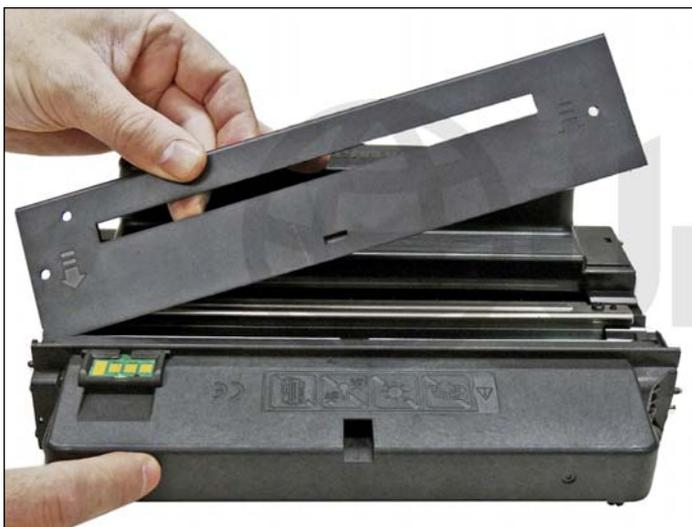
7. Separate the two halves slightly and lift off the middle top cover.
