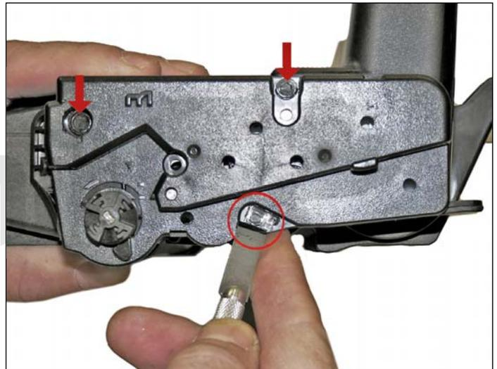
2. On the opposite side end cap, take the chisel blade knife and slice off the heads of the three plastic rivets. See previous step for recessed rivets. Leave the end cap on for now.
