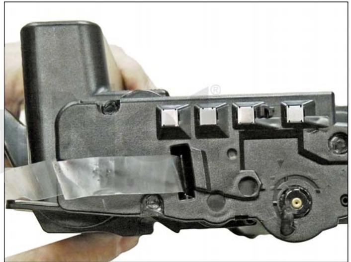
40. Clean the contacts on the left side end cap, and replace the conductive grease.
