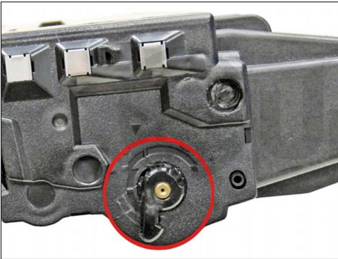
3. The drum axle arms on both sides of the cartridge stay with the end cap. There is no need to remove them.
