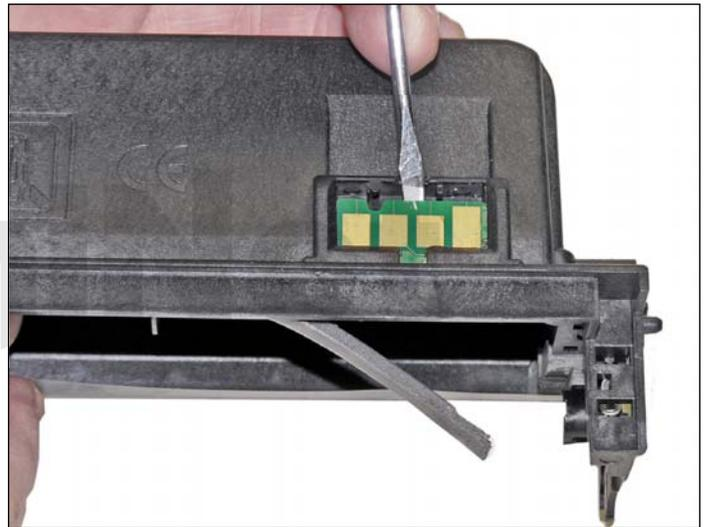
15. Lift up on the tab as shown, and press the chip out through the opening.
