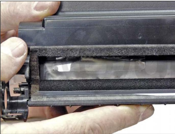
29. Install the seal when available through the developer roller opening.
