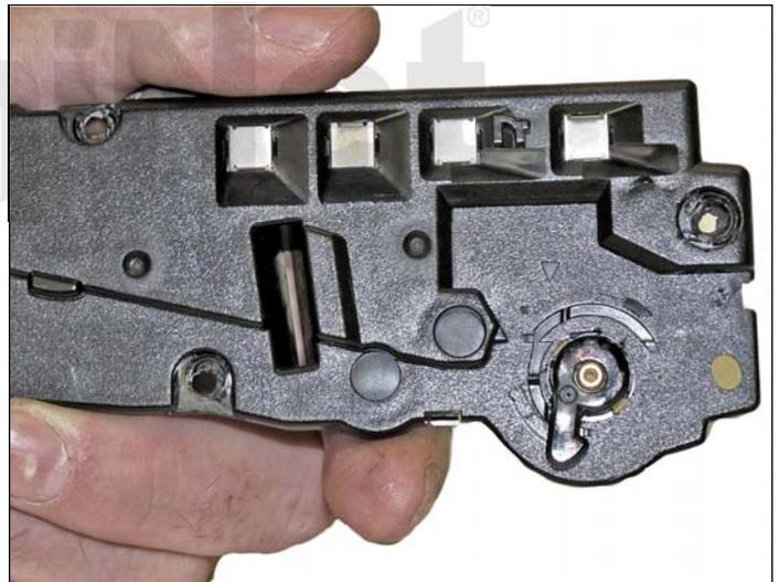
6. On the right side end cap, press in on the three tabs and remove the end cap.
