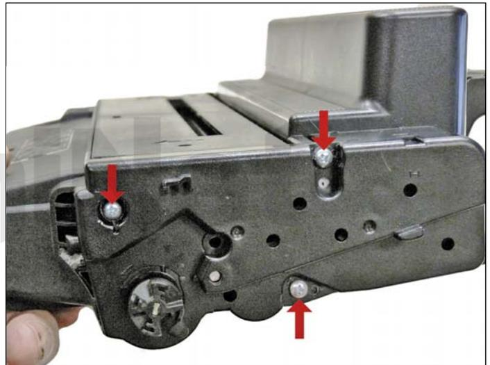
43. Drill three small holes that correspond to the screw size you are using.
