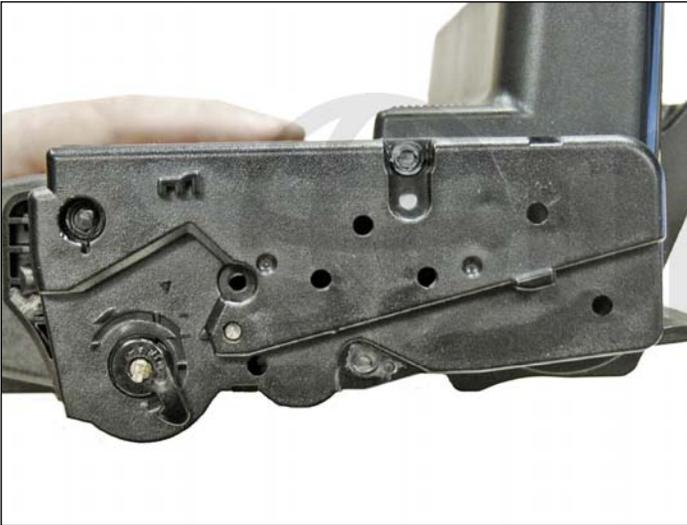
42. Clean the hubs on the gear side or right side end cap.
