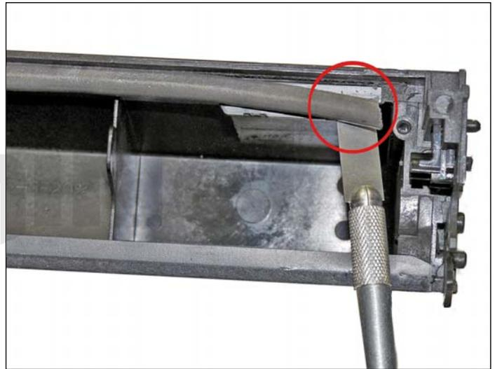
13. Carefully remove the wiper blade seal from the right side (chip side). Peel the seal back around three inches.
