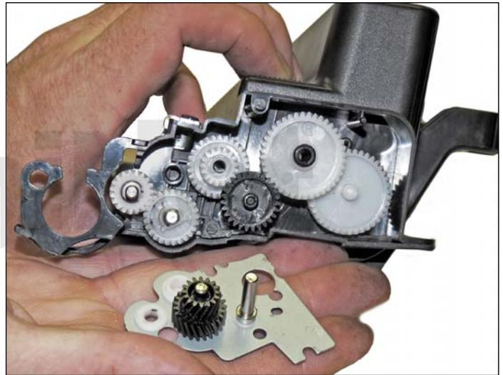
36. Install the gears in the order as shown.
