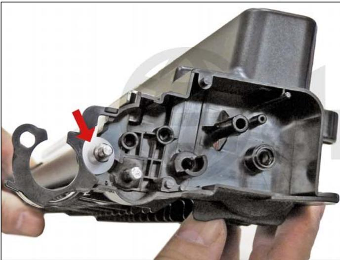
35. Replace the bushings on both side of the developer roller.
