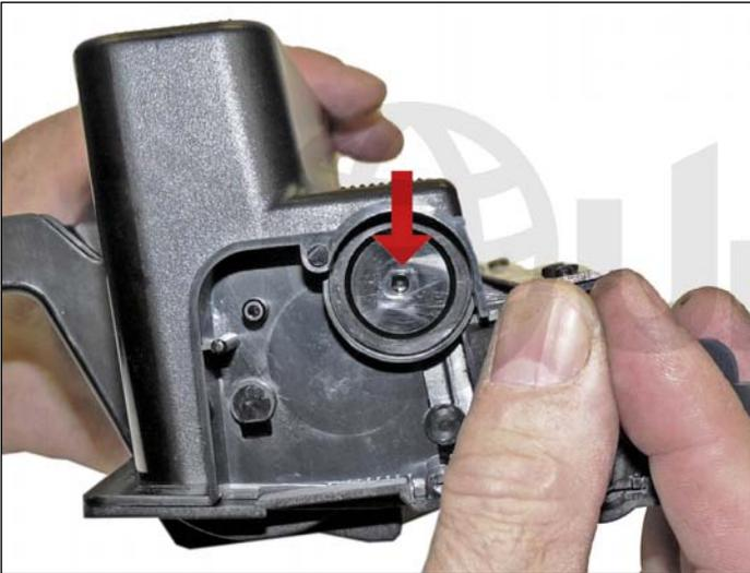
22. On the supply hopper, carefully pry out the fill plug and dump out any remaining toner. The fill plug can be difficult to remove as it is recessed. Take a small common screwdriver and work it around the edge, lifting slightly until it comes loose.
