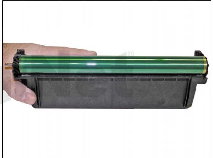
21. Install the drum into the waste hopper, with the large gear of the drum to the gear side (non-chip side).
