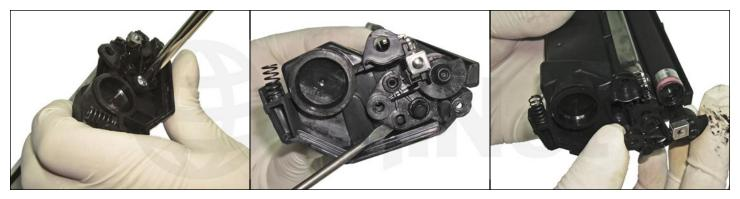
15. At the opposite end, remove the screw holding the contact end plate. It must be noted that there is NO conductive spring or blade doing the electrical work. Instead, a conductive plastic tip at the plate can be found. This is further confirmed by the use of fair amount of conductive grease both at this bearing and the inside of the metal developer roller.
