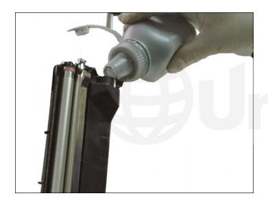
23. Fill the hopper with dedicated toner for use in MLT-D101, and place the filling plug back to close the hole. Check for leaks.
