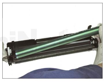
7. Slide the OPC drum axle out just enough to allow the opposite end of the drum to be lifted out of position and remove it.
