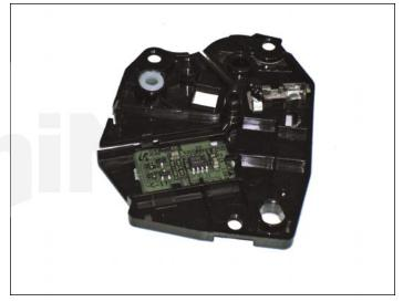
5. Proceed now to remove the screws of the end cover on the right (contact side) and pry open with the small screwdriver at different consecutive points until separation is accomplished. Even though the cover seems to be formed by two sections, it is a unit with a rather thin centerpiece. Worth noting also the way the chip is internally held and the need to be replaced prior to reinstalling the cover.
