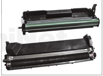
6. Repeat the removal of the left end covers in its two parts, starting with the top one and then the lower one.
