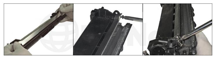
20. Install the doctor blade in its place, securing it with the proper screws.
