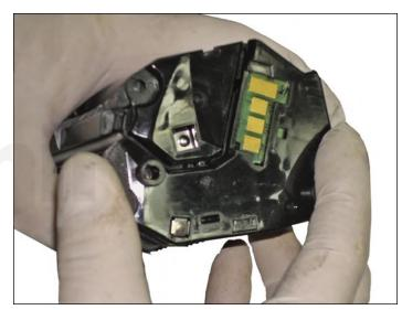
26. Work on the opposite end by taking the end cover and lubricating all contact points, and replacing the chip as shown.
