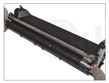
16. Slide the developer roller out and be particularly careful with both plastic bushings acting as separators at each end of the roller. Clean the roller with a soft cloth and use isopropyl alcohol if needed, to remove all traces of dirt and grease from the surface. Replenish with conductive grease as needed.
