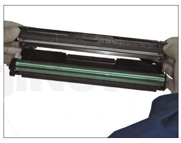
24. Now take the image section and place it on top of the developer section as shown, positioning the compression springs properly.
