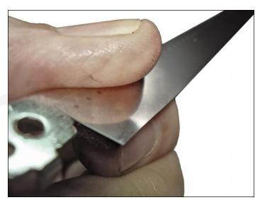
18. Remove the two Phillips screws and doctor blade from its place, then clean with a soft cloth.
