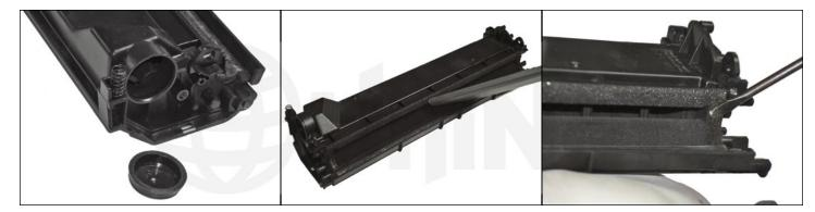
19. Vacuum the hopper completely, including the feed roller, and remove the fill plug to facilitate the work.
