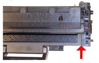
31) If your cartridge has a fuse, it needs to be replaced. Replace the fuse located on the right front of the cartridge (with the handle away from you. The ML-2010 does not use a fuse, and no other machines/cartridges are available yet (9/2005), but the slot for a fuse is there so it is possible that some of these cartridges will use one. See **Figure 34**
