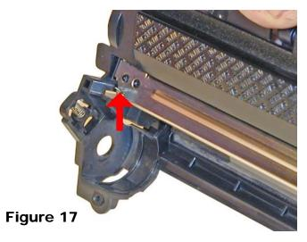
It is highly recommended that the Doctor Blade be cleaned. Failure to do so will cause streaking. Dampen a cotton swab with alcohol, and clean the blade. Be careful not to press too hard and damage the blade. If the blade has a heavy buildup of toner on it, clean it with Acetone, and then alcohol.
