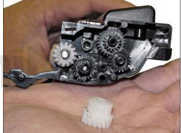
29. Install the gears as shown.
