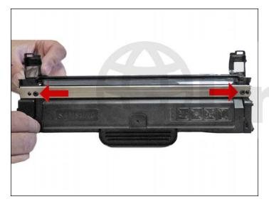
23. Remove the two screws from the doctor blade, and remove the blade. Clean out all the remaining toner from the hopper.
