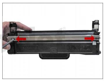
26. Install the doctor blade and two screws.
