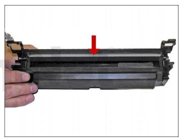
24. Make sure the doctor blade sealing foam and the developer rollers seals are clean and intact.
