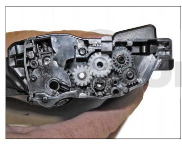
5. Remove the gears.
