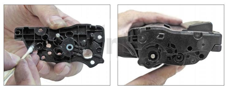
35. Clean the hubs on the gear side end cap, and replace the conductive grease.
