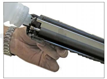
28. Fill the hopper with toner for use in Samsung ML-2525.
