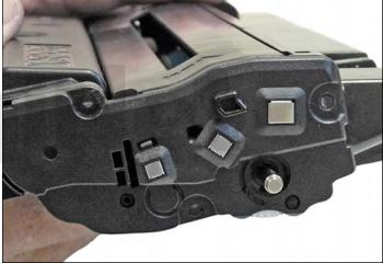
32. Clean the contacts on the left side end cap, and replace the conductive grease.
