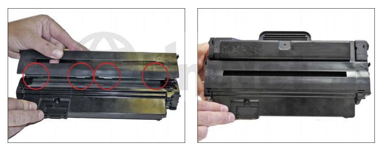
31. Slide the middle top cover/PCR assembly into place.
