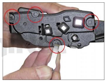
2. On the left side end cap take the chisel blade knife and slice off the heads of the four plastic rivets.
