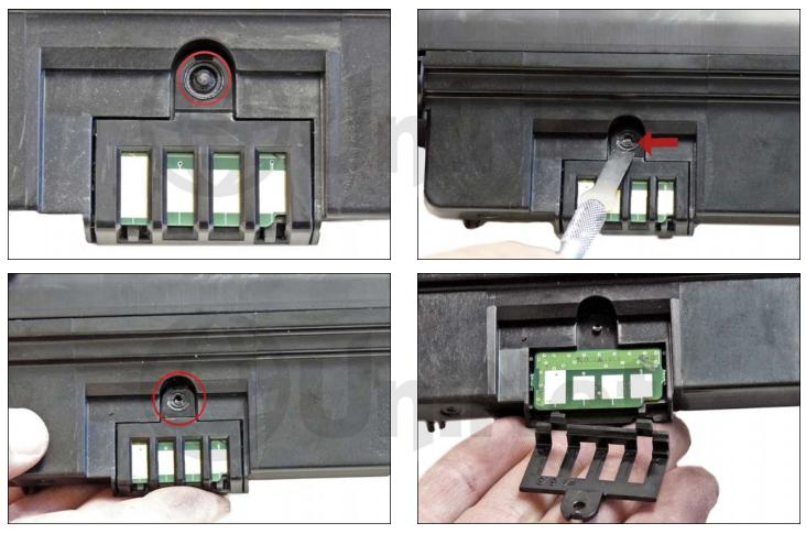
38. To replace the chip, slice the top of the plastic river off with the chisel blade knife.
