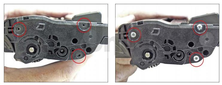
36. Drill three small holes that correspond to the screw size you are using.
