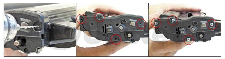
33. Drill four small holes that correspond to the screw size you are using.
