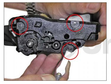
1. Place the cartridge with the handle up, facing towards you. With the chisel blade knife, slice off the heads of the three plastic rivets. Leave the end cap in place for now.
