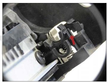
16. Install the two PCR holders. There are slots in the holders that fit over tabs in the cartridge.
