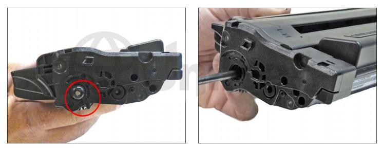
3. Remove the drum axle arm from the right or large gear side of the cartridge.
