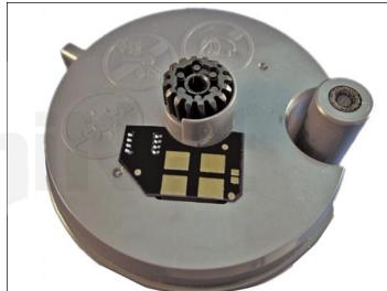
5. The OEM chip is not removed. A new chip is placed over it.
