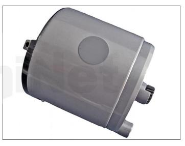
4. Cover the hole using a small piece of tape. Make sure the seal is tight and that there are no leaks. Also make sure the tape/label does not extend to the top of the cartridge as it is installed, this area has a very tight fit and the seal may be torn off as the cartridge is installed.
