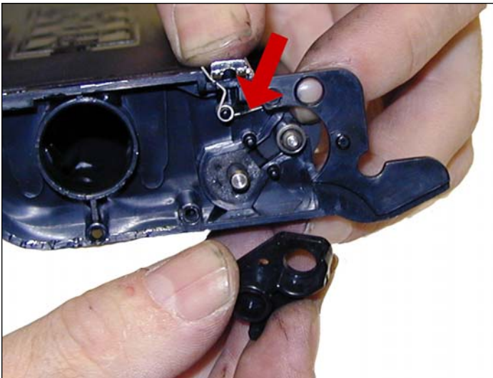
28. While holding the DVR contact spring back, install the double bushing. Make sure it snaps into place.
