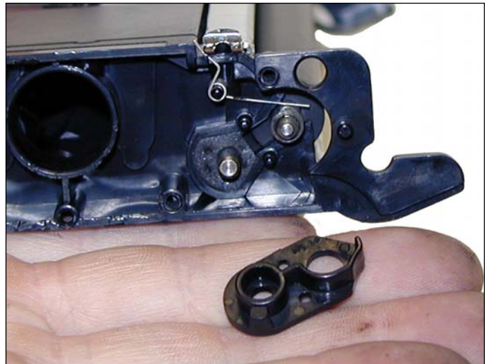
21. Press in on the bushing tab, and remove the bushing. Be careful not to lose the spring.
