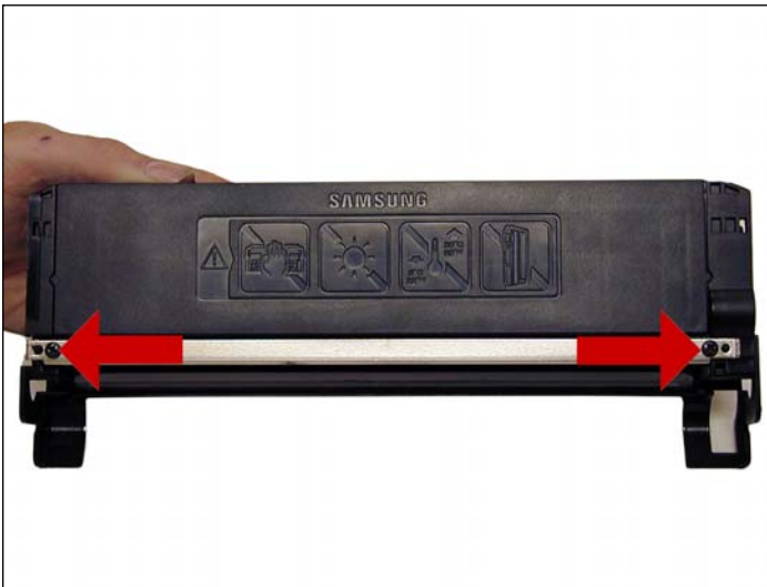
26. Install the doctor blade and two screws.
