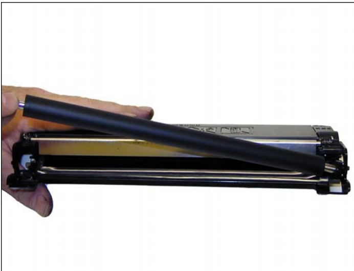
22. Slide the developer roller over, and lift out to remove.
