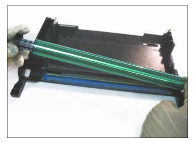
**REMOVING THE OPC DRUM** 26. Remove the OPC drum as shown.
