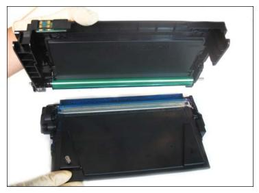
6. Separate the two halves as shown.
