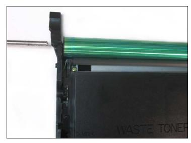
25. Follow through until the axle is completely removed.
