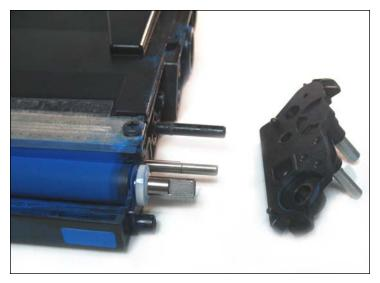
16. Gear-side support plate (shown) removed.
