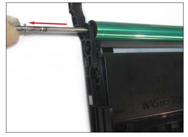
**REMOVING THE DRUM AXLE** 24. Pull out the drum axle through the opposite side as shown.
