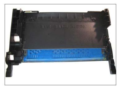
30. Clean thoroughly and reassemble the drum unit.
