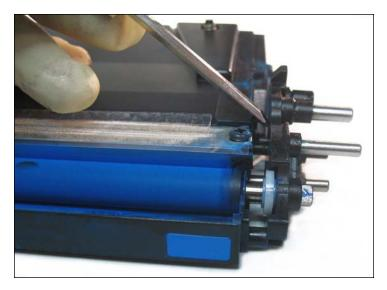
15. Using a flat head screwdriver, pry the loosed plate away from the cartridge to remove it completely.
