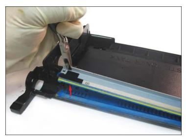
29. Using a pair of pliers, grip and remove the wiper blade as shown.
