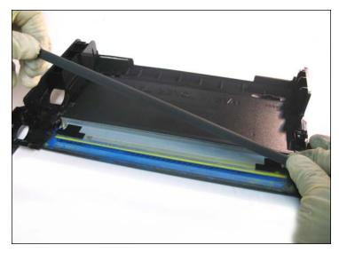
**REMOVING THE PCR** 27. Remove as shown.
