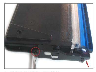
**REMOVING THE CONTACT END PLATE** 8. First, remove the end plate by removing the two screws (shown) that hold it in place.
