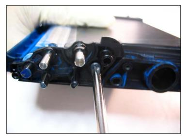
**GEAR-SIDE SUPPORT PLATE REMOVAL** 14. Locate the gear-side support plate (shown) and remove the screws that hold it in place.
