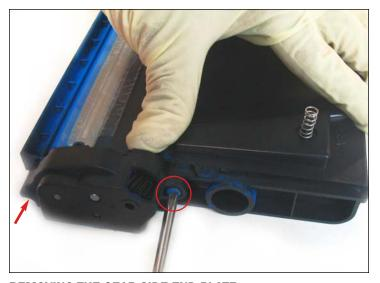
**REMOVING THE GEAR-SIDE END PLATE** 10. Remove the two screws that hold the end plate in place. This will allow access to the gears inside. Remove the first screw from the area shown.
