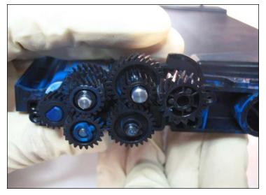
**REMOVING THE GEARS** 12. Remove the gears.
