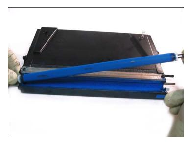
19. Remove the developer roller as shown.
