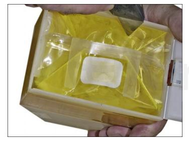
3. Cut a small incision on the plastic bag that will allow you to clean out the old toner and to fill it again. This slit will be sealed with tape when done.
