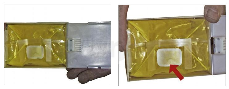
2. Once you release the clips, the cover can be lifted revealing the toner bag.
