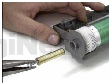
2. Pull until the drum pin is completely out.
