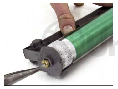
1. Insert a small screw into the drum pin hole shown, turning it clockwise until it anchors in place. Using a pair of needle-nose pliers, grasp the exposed portion of the screw.
