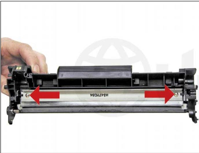
8. Coat the new/cleaned wiper blade with your preferred lubricant. Install the wiper blade and two screws.
