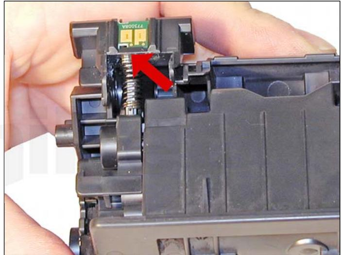
26. Set the hopper tension springs back in place.
