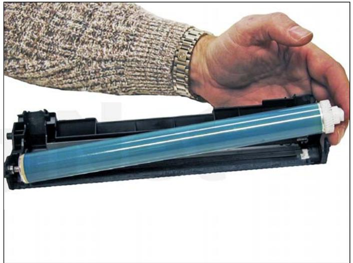
11. Install the new/cleaned drum hub side first.
