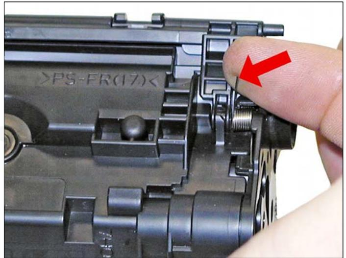
27. With the drum cover spring as shown on the end cap, install the end cap.
