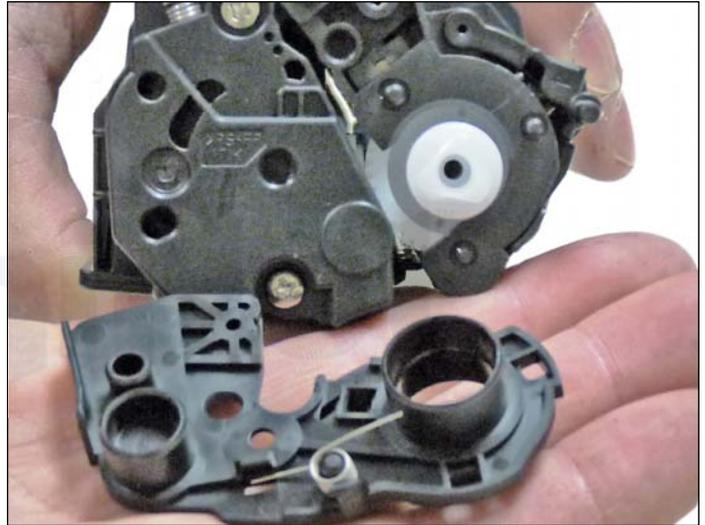
1. With the handle facing you, remove the right side screw and end cap from the cartridge.
