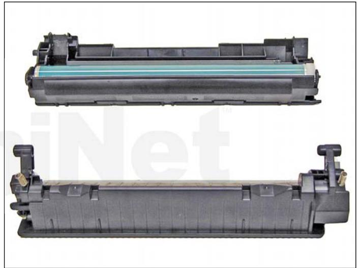
3. Slide the waste/drum section over to the left side.
