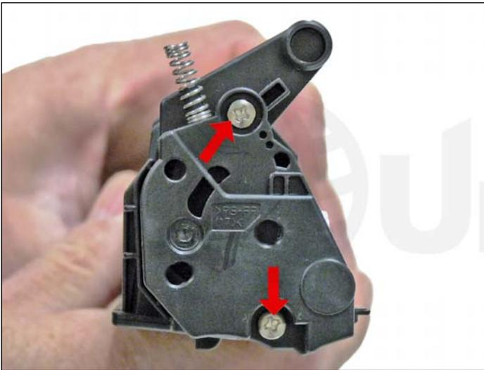
12. On the toner supply chamber right side, remove the two screws and end cap.
