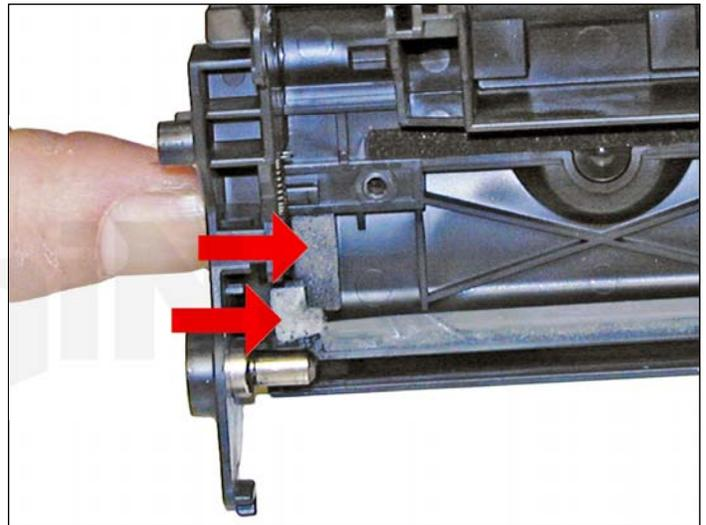
7. Clean out all the waste toner from the hopper. Be careful not to damage the recovery blade located next to the wiper blade.
