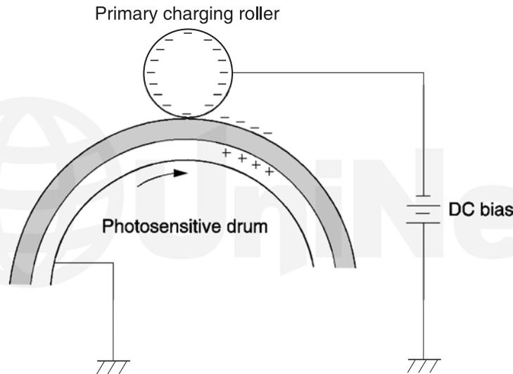
The image formation process consists of a series of steps. In the **first step**, the Primary Charge Roller (PCR) places a uniform negative DC Bias voltage on the OPC drum surface. The amount of the negative DC Bias placed on the drum is controlled by the printer intensity setting. This process is part of the Latent Image Formation Block.
