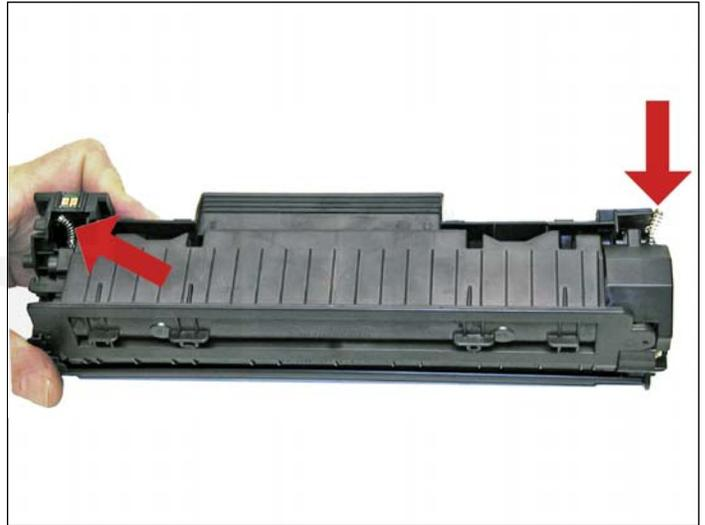
2. With the pair of needle nose pliers, release both the hopper tension springs.
