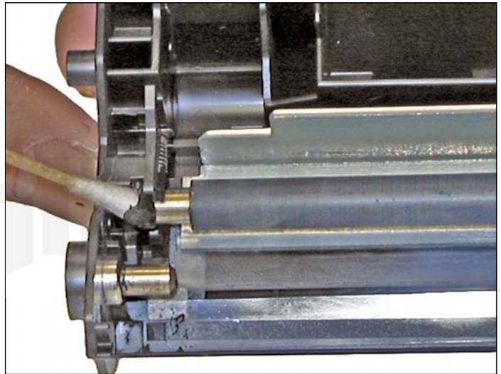
9. Install the cleaned PCR. Place a small amount of conductive grease on to the black holder side of the shaft. Just a small amount of grease is more than sufficient.
