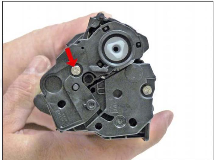
28. Lift up the drum cover spring tail to fit as shown on the drum cover.
