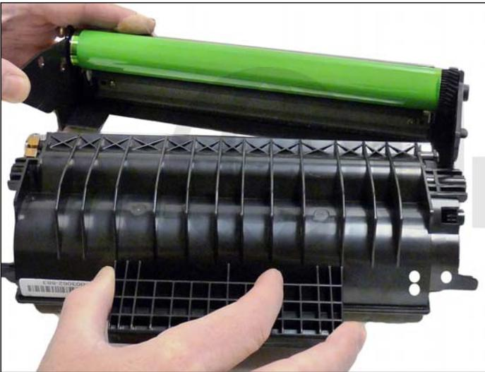
3. Pry out one of the side panels, and separate the two halves.
