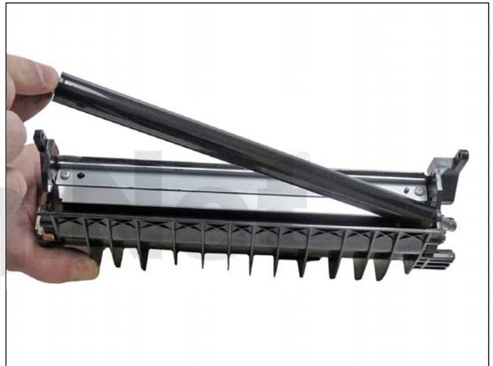
18. Pry off the metal bushings from both sides of the developer roller shaft.
