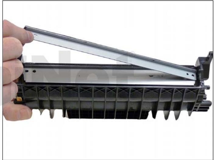
21. Remove the upper metal brace, being careful not to damage the alignment pins. The pin on the left side is normally tight so more care should be taken there.
