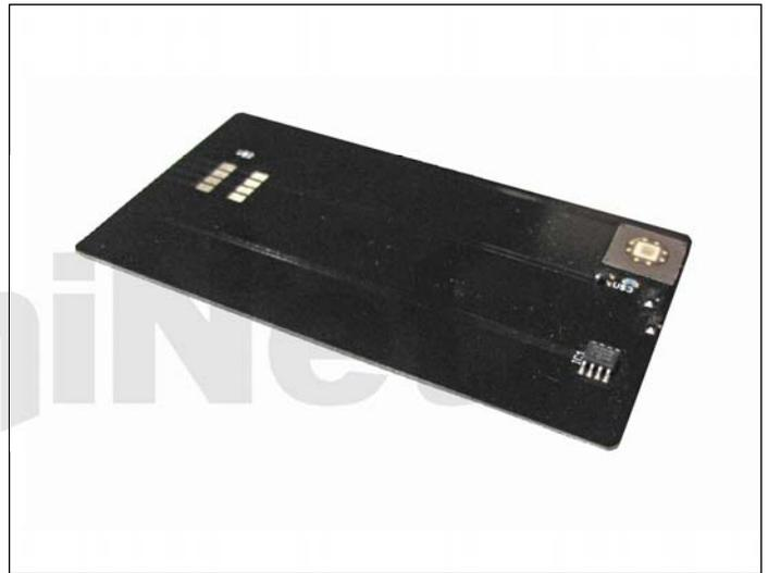
37. After the cartridge has been tested and bagged, tape the key card to the top of the bag so the user will see it. This key card is installed into the printer separately from the cartridge.
