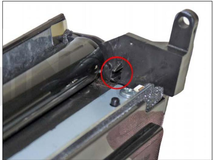
17. Remove the screw, holder and contact from the contact side of the developer roller.
