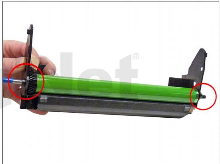
4. From the gear side of the drum-half, take a small punch (1/4") or screwdriver and drive the metal axle pin out. This axle is fairly tight. Make sure you do it from the gear side, (the keyed side). If you try and drive the axle out from the opposite side, the axle will not move and you may damage the drum ground contact inside the drum. Remove the drum.
