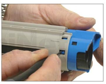
2. Press down on the locking tab of the blue handle. Rotate the handle to open the toner port. Vacuum/blow out any remaining toner.
