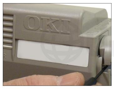
3. Carefully pry off the gear cover with a small jeweler's screwdriver.
