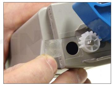
4. Cut the waste hopper seal just past the small white gear.
