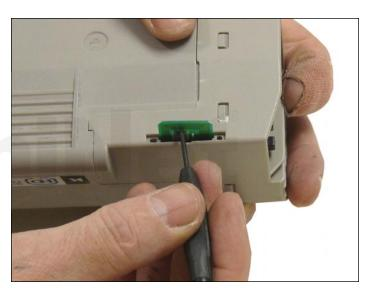
8. Remove the old chip and install the new. Be sure to keep the component side up when replacing the chip.
