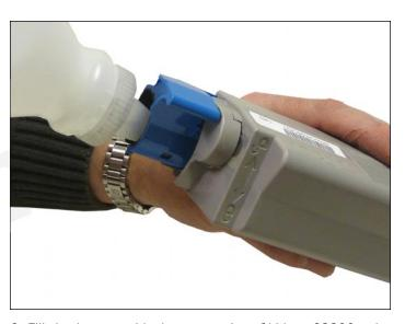
6. Fill the hopper with the appropriate Okidata C8800 color toner. Replace the fill plug.
