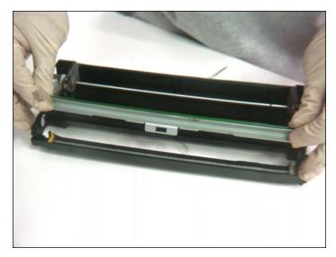
18. Remove the wiper blade as shown.
