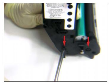
9. Remove the two screws that hold the end cap (gearless) in place as shown.
