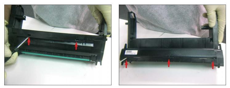
5. Use a small flathead screwdriver to push in the five tabs located on the back and front of the cartridge to unlock the drum unit cover.
