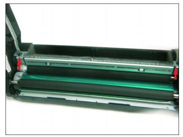
7. Remove the two screws that hold the doctor blade in place as shown.
