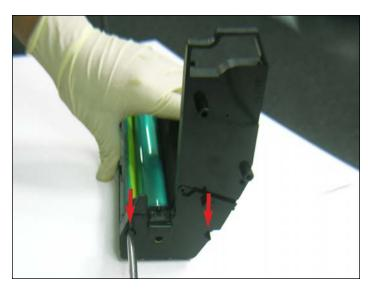
13. Remove the screws on the remaining end cap (gearside) that hold it in place.
