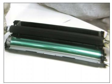
15. Remove the developer roller as shown.
