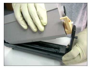
3. Lift the hopper from the drum unit, starting from the blue handle side as shown, then set aside.
