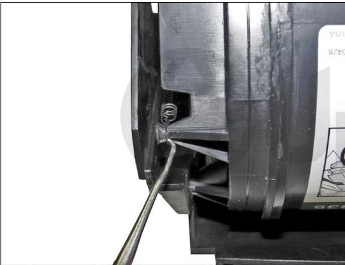
8. Make sure the bottom edge of the OEM toner hopper is parallel to the OPC drum. If this edge is NOT parallel, then one of the white wheels is not properly locked in place or one of the shipping lock pegs is not in the conversion cover hole.
