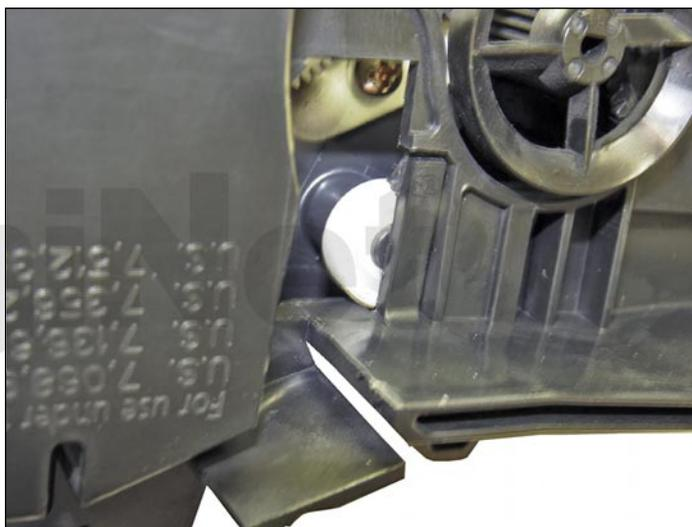
6. On the opposite side of the conversion cover, pull the right side wall out with one hand and use your other hand to snap the OEM hopper in place until the white wheel clicks and locks under the retaining hook. On the backside, make sure the shipping lock peg fits into the hole on the conversion cover.
