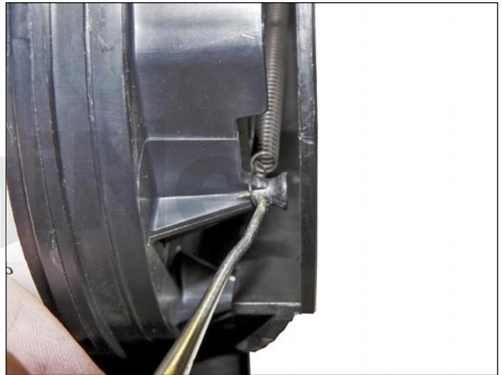
7. Using a spring hook, Install the two springs from the universal conversion cover to each side of the OEM toner hopper.
