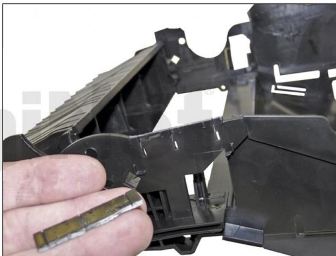
1. **IMPORTANT:** Before starting, take a pair of pliers and break off the side plastic tabs as shown. If this is not done, the plastic will block the electrical contacts on the toner hopper from making contact with the printer and print defects will result.
