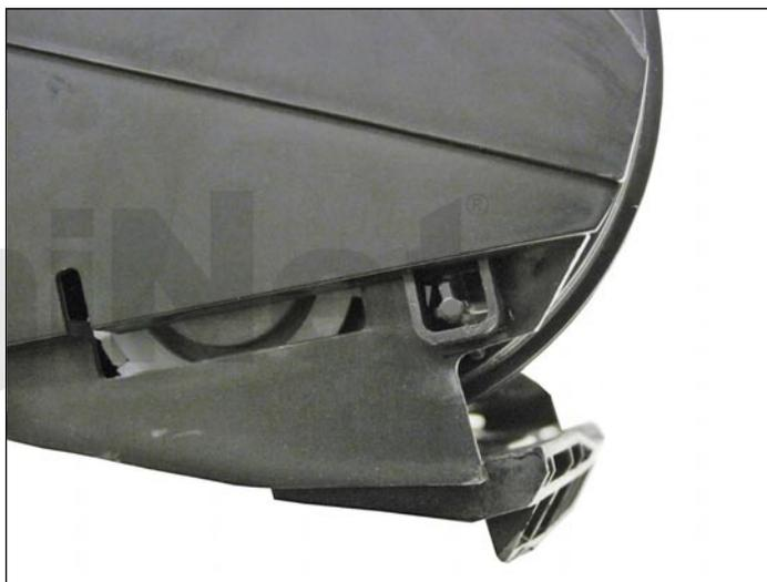
5. Slide the left side of the OEM toner hopper into the universal conversion cover. Make sure that the white wheel slides under the retaining hook of the conversion cover and that the shipping lock peg of the OEM toner hopper fits into the hole on the conversion cover.
