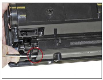
2. Make sure the toner port is closed. If open, close the port by turning a tab on the gear with a screwdriver.
