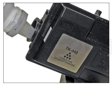
3. Fill the cartridge with toner for use in the TK-342 series of cartridges. Use a Samsung CLP-300 seal to cover the hole you drilled.
