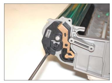
12. Remove the two small black screws from the drum contact plate.
