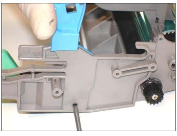
10. Note there are two screws on each side of the cartridge.
