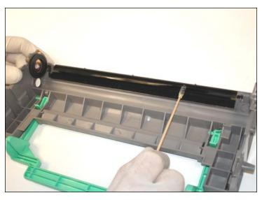
18. Clean the recovery blade with another cotton tip swap with alcohol isopropyl. Be careful to don't damage or bend the blade. Otherwise it would cause spotting.
