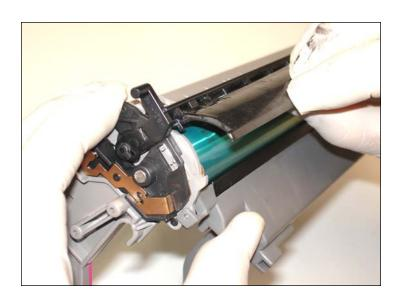
7. Release the drum shutter from the hopper.
