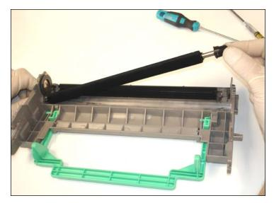
15. Remove the PCR by lifting it from the right side of the drum unit.
