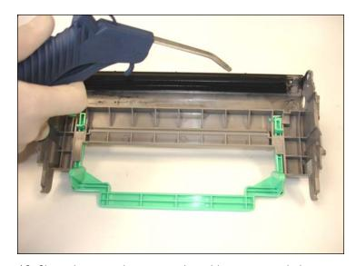
16. Clean the waste hopper section with compressed air.
