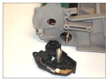
13. Notice the contact bar in the inside part of the plate is released placed in the black plastic end cap housing. Otherwise, keep it aside.
