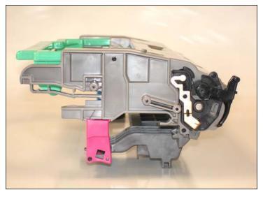
6. Contact side view of the drum unit. Where the pink plastic fixing arm is located.
