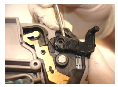
8. Remove the shutter arm from the plastic pin with a small flathead screw driver.
