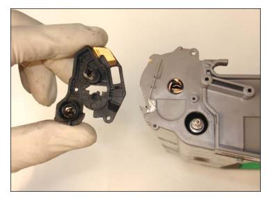
24. Lubricate the electrical contact as done previously. NOTE: Don't forget to place the little silver contact bar.
