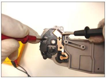
26. Check the electrical continuity with a tester to ensure good contact between both parts of the contact end plate.
