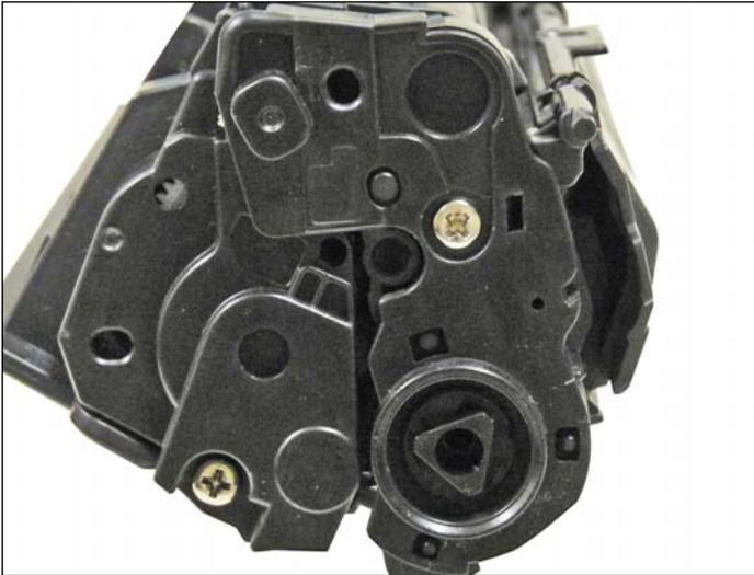
9. Install the wiper blade, PCR and drum back into the waste hopper. Re-assemble the two halves and install the new drum bearing plate supplied with the kit. The conversion is complete!
