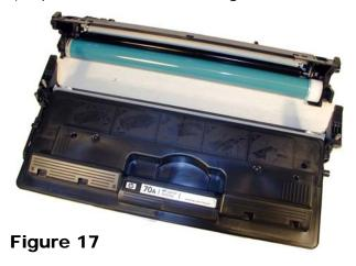
5) On the Waste section, take a common screwdriver and remove the Metal Axle pin/spring loaded cover located on the right side of the cartridge. This is the same type of drum axle pin that the 2400 series uses. It comes out easily enough, but be careful as it seems somewhat fragile. See Figures 18 & 19
