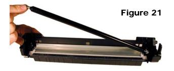
8) Remove the wiper blade and 2 screws. See Fig. 22
