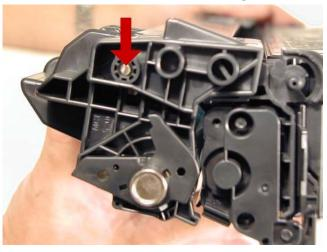
32) Install the spring in the drum cover arm as shown. Install the metal bar into the hole and slot. Install the arm. See **Figures 51 & 52**
