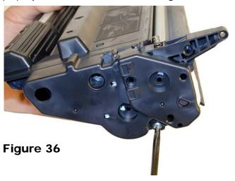
19) Take the Dremmel tool again and cut away the recessed plastic rivet do not grind through the end cap! To separate the end cap from the cartridge, take a common screwdriver, pry up the end cap and slide the screwdriver against the shoulder. Press the screwdriver against the shoulder until it snaps free. Do the same for the small rivet. See **Figures 37, & 38**
