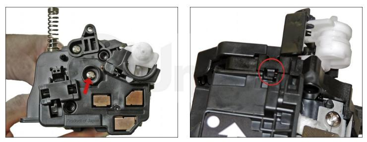
26. On the opposite side end cap, remove the single screw and press in on the tab to release it.
