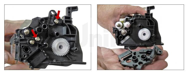
24. Remove the two inner screws, and inner gear end cap.
