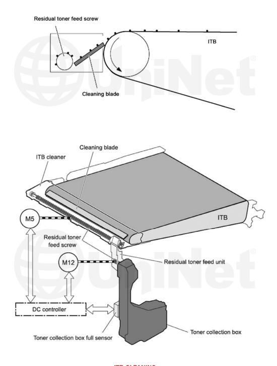
ITB CLEANING The ITB is cleaned by the ITB cleaning blade.
