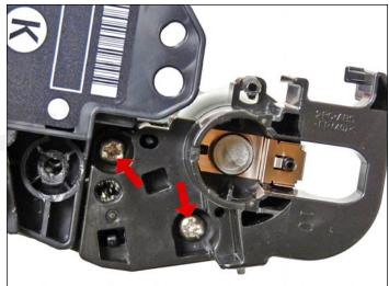
19. Install the contact end cap on the right or label side of the chamber.
