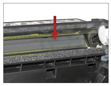
34. Install the seal onto the seal rails. Pull the release tape off one inch at a time and press the seal in place as you go.
