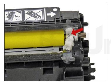
38. Press the developer roller seal back in place.
