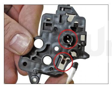
40. Clean the contacts and replace the conductive grease on the contact end cap.
