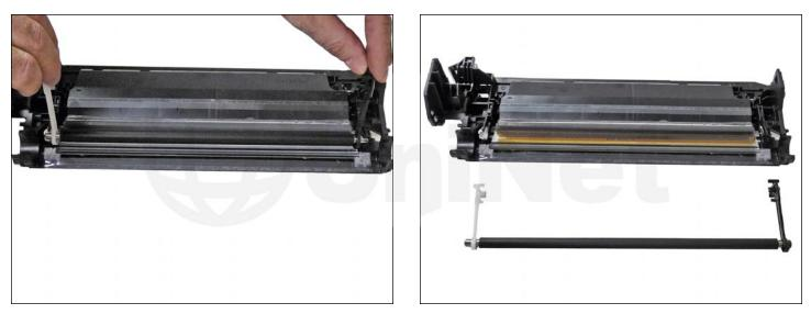
10. Remove the PCR by lifting up on the black and white PCR locking arms.
