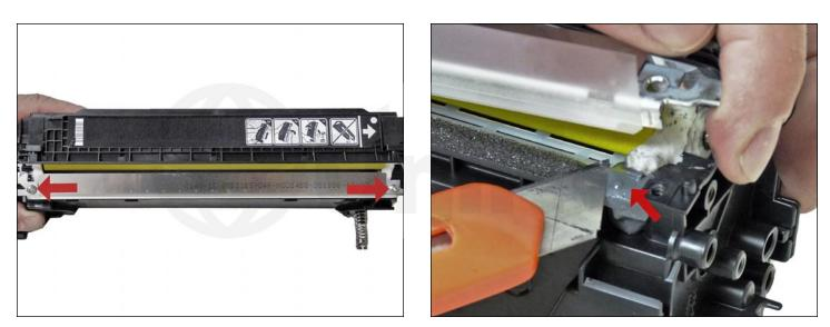
28. Remove the two screws from the doctor blade and start to lift the blade up.
