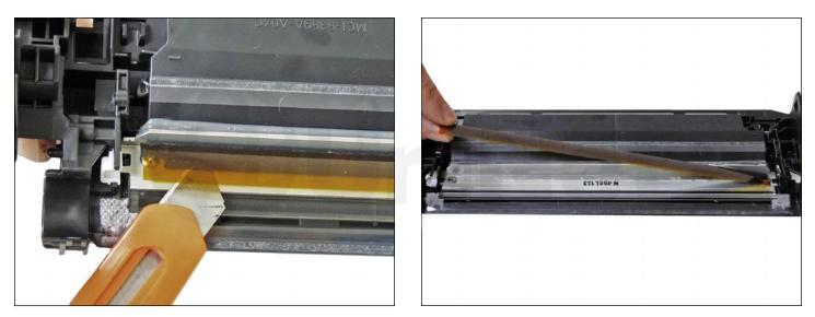
11. To remove the wiper blade, the amber film assembly needs to be removed.
