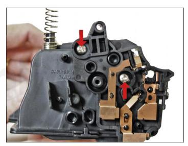
41. Install the contact end cap and two screws.
