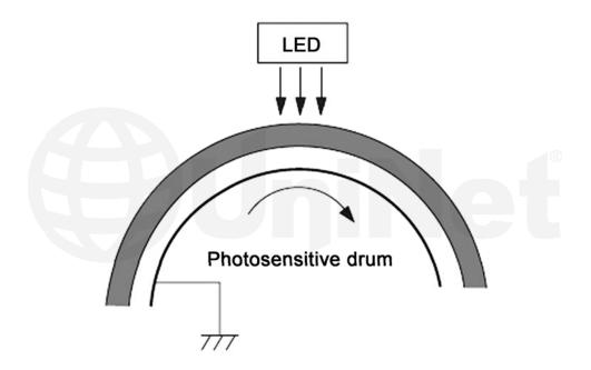
In the first stage, light from the pre-exposure LED strikes the drum to remove any residual charges from the drums surface.
