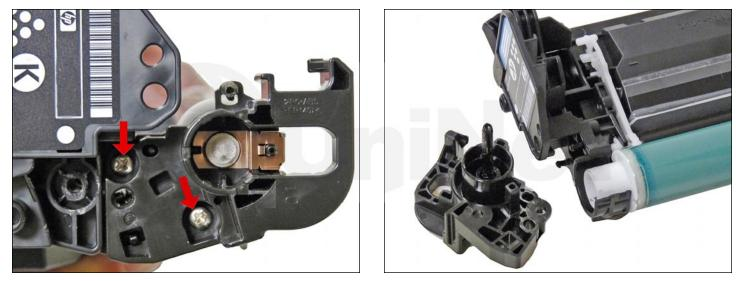
8. Remove the two screws from the contact side end cap.
