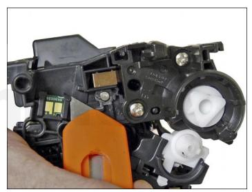
50. Remove the chip by cutting the plastic off the edges of both side of the chip.
