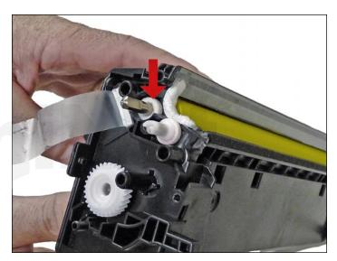
37. Install the feed roller felt washers.
