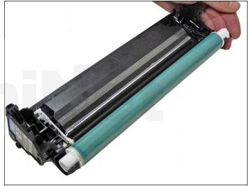
18. Install the drum, short hub side to the right (or label side) of the chamber.
