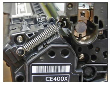
1. Remove the spring from the label side of the cartridge.
