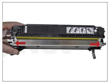
39. Use the appropriate shims and install the doctor blade and two screws.
