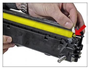
36. Install the feed roller and bushing.
