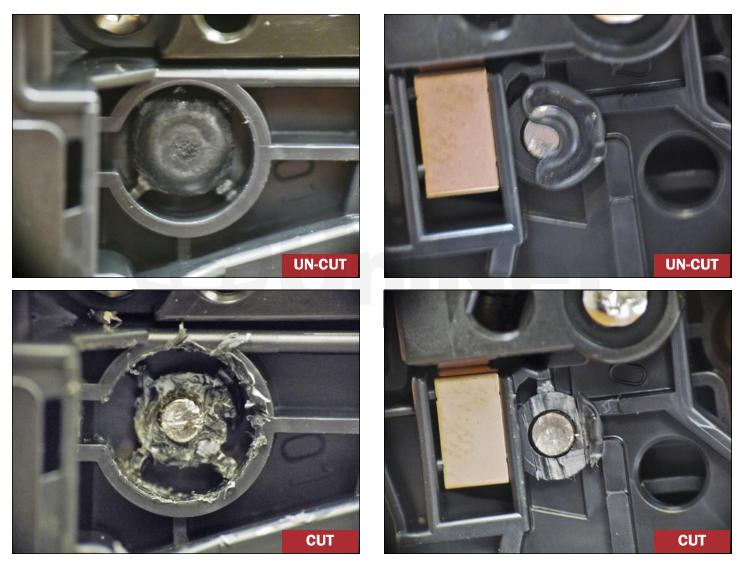
2. With a razor knife, carefully shave the plastic from the heads of the hinge pins.
