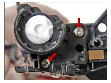
20. Install the opposite side end cap and two screws.
