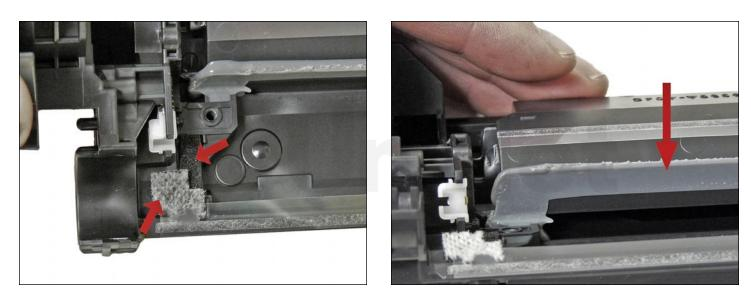
14. Clean the felt seals on each end of the wiper blade. If the wiper blade glue has toner on it, clean it off with alcohol and a foam swab. If it does not become sticky again, it needs to be removed, and a good silicone caulk used to seal the blade off. GE 100% Silicone and Phenoseal are two good brands for this.
