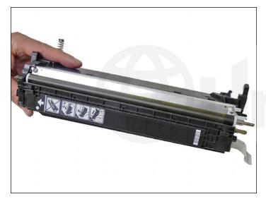
42. Install the cleaned developer roller (do NOT use any chemicals to clean this; a lint-free cloth works fine).
