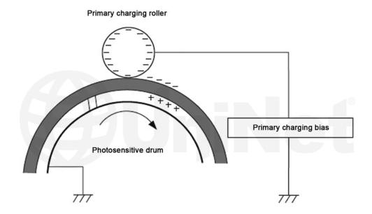
Then, the primary charge roller (PCR) places a uniform negative DC voltage on the OPC drum surface.
