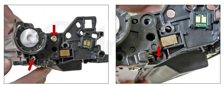
7. On the waste chamber, remove the two screws from the drum gear end cap.
