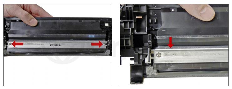
15. Install the new wiper blade and two screws.
