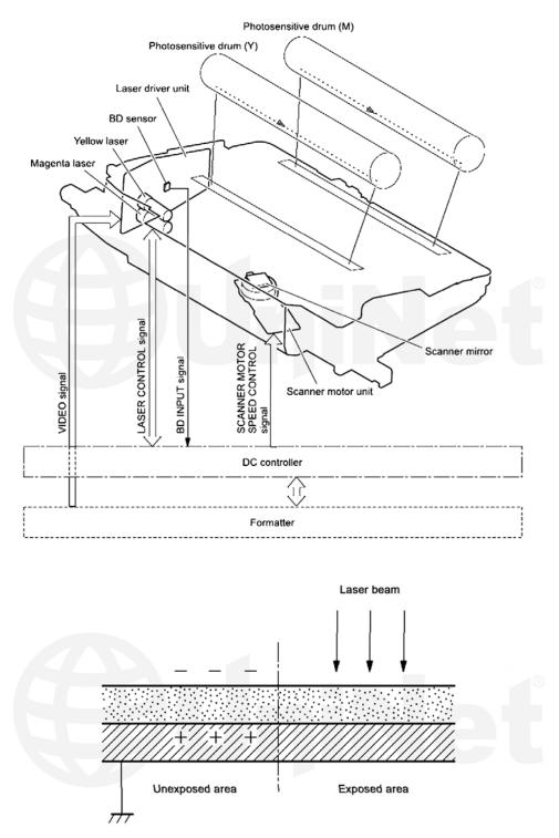
In the **second** stage, the laser beam is fired onto a rotating mirror (called the scanner). As the mirror rotates, the beam is reflected into a set of focusing lenses. The beam then strikes the drums surface, reducing the negative charge and leaving a latent electrostatic image on the drum. The areas where the laser did not strike the drum will retain the higher negative charge.
