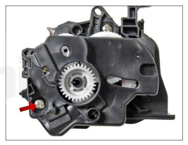
21. On the supply chamber, remove the outer screw from the gear side end cap.
