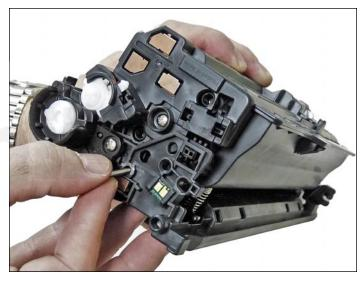
48. Install the two pins, small pin to the gear side of the cartridge.
