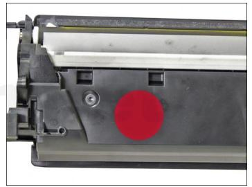
If you wish to make it easier to seal, a hole can be cut in the flat side of the chamber. Install the seal, and then fill through the hole. Make sure you cover the hole with a good quality seal!
