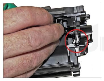
47. Place the two halves together, contact side first. On the gear side, snap the lock in place.
