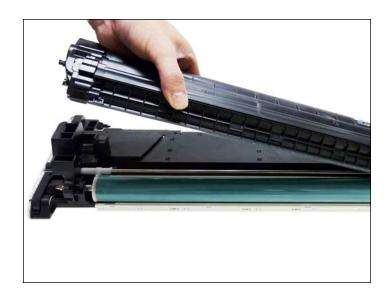
6. Lift the developer unit off the cartridge.
