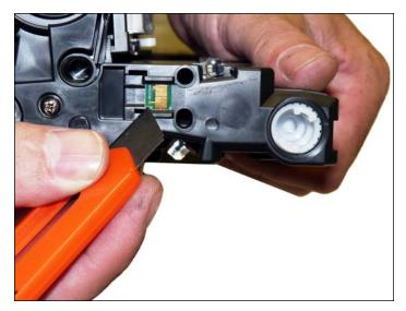
40. Replace the chip by slicing the melted plastic from the top edge. Slide the chip out and replace. Lock the replacement chip in with two small dots of hot glue.
