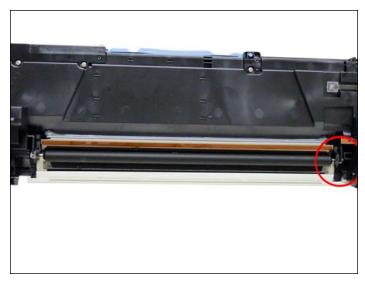
22. Clean the PCR and install the PCR assembly. Be careful not to damage the film. Replace the conductive grease on the black holder side of the PCR.
