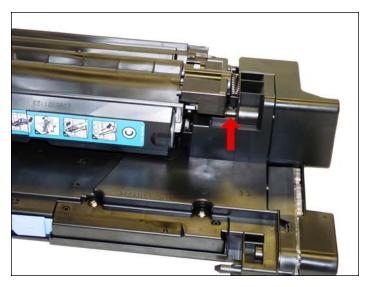
38. On the gear side, install the small metal pin in the end cap.
