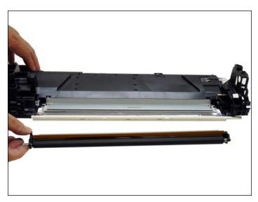
16. Remove the PCR assembly. The film will come with it.
