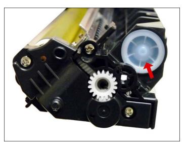
36. When developer is available, remove the fill plug, dump the old developer vacuum the chamber out and install the new developer. At this time we do not recommend the doctor blade be disturbed.
