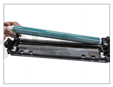
16. Install the drum (short hub side) onto the long drum ground/axle pin. Make sure there is conductive grease on the drum ground/axle pin.
