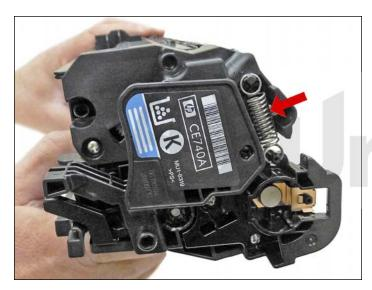
1. The pins in these cartridges are stepped. In other words the outside is thicker than the inside. To remove the pins, you must carefully shave the plastic away from the pins.
