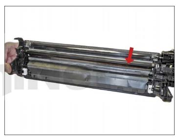
14. Clean the PCR with your preferred cleaner and install in the cartridge with the PCR holders. Make sure you lock the locking arms in place.
