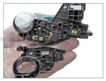
6. On the waste chamber, remove the two screws from the drum gear end cap.
