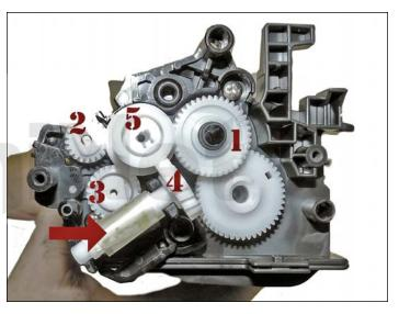
42. Install the gears in the order shown. If you installed a seal, slide the seal end through the take up gear and wrap the loose tail tight on the roller.
