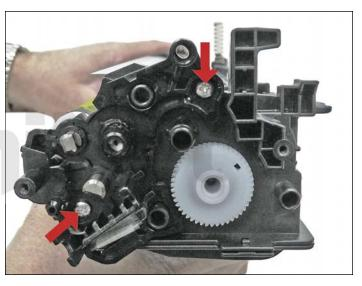
24. On the gear side inner end cap, remove the two screws and end cap.
