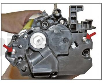
18. On the supply chamber, remove the two screws from the gear side end cap.  $\,$
