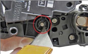
2. With a razor knife, carefully shave the plastic from the heads of the hinge pins on both sides of the cartridge.
