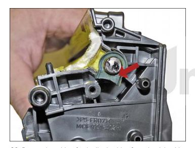
30. Pry out the rubber feed roller bushing from the right side.
