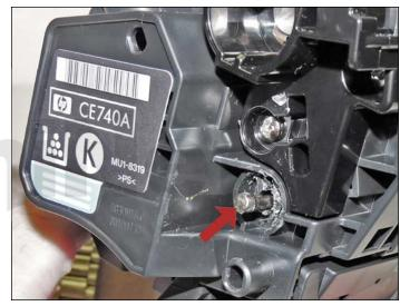
3. Remove the pins with flush cutting wire cutters.
