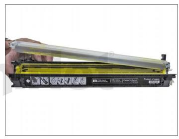
27. Remove the two screws from the doctor blade and start to lift the blade up.
