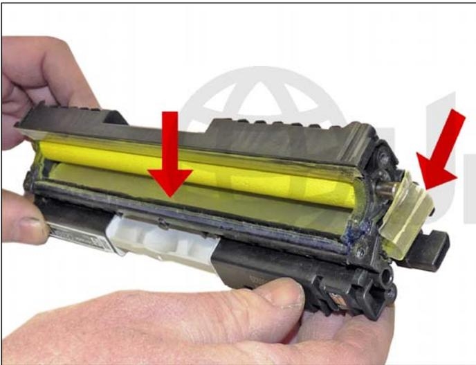
11. If you are using a seal, install it now. Make sure the tail of the seal comes out through the seal plug hole.
