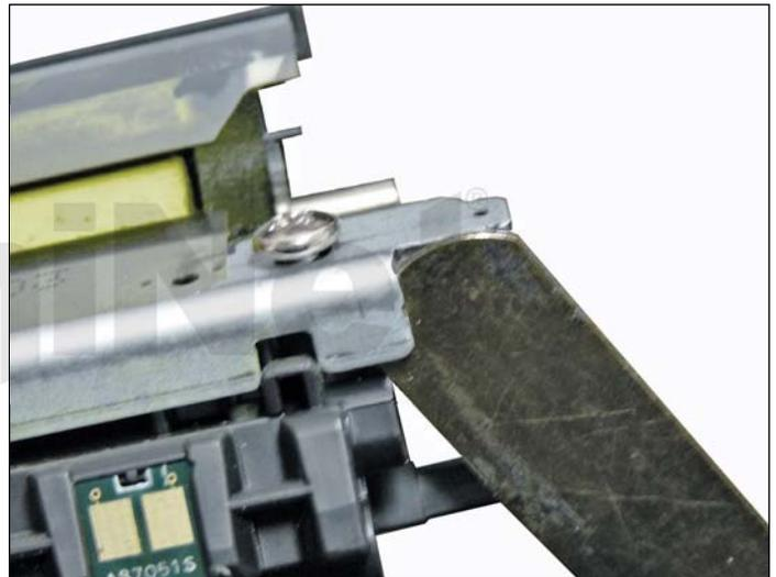
13. Install the doctor blade and two screws. **NOTE:** The doctor blade must be gapped for the cartridge to work properly. Use either doctor blade shims, or set the gap manually to 1.8 mm. The doctor blade gap is set from the back 90-degree edge of the blade, not the top or screw side. In other words, the gap is to set the distance of the edge of the doctor blade to the developer roller - NOT the height of the blade.
