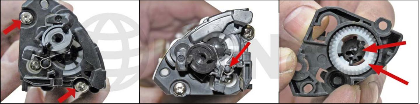
2. On the gear side of the cartridge, remove the two screws from the black plastic end cap. Note the spring loaded drive gear.
