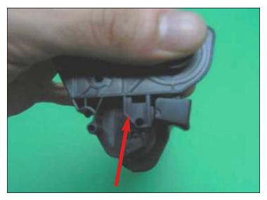
8. Add a drop of glue in area shown, then place the trigger arm as shown on the photo
