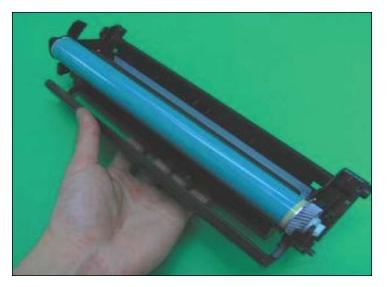
**INSTALLING THE OPC DRUM** 3. First, place the Drum into the Waste Hopper as shown.
