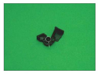
**INSTALLING THE PCR CONTACT TRIGGER** 7. Install the PCR contact Trigger onto the P2015 Waste Hopper as shown in the following steps. This trigger is included in the P2015 Conversion kit.
