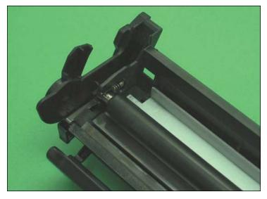
2. Install the PCR as shown. If you are using an OEM PCR, please make sure it is carefully cleaned.
