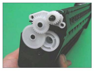
15. Install the Mag Roller as shown in the Hoper as shown in the photo. Then insert the Right Stabilizer, and all drive gears on the right side of the hopper.
