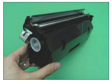
10. Fill Hopper with toner and insert the filler cap.
