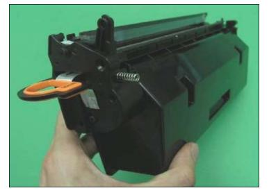
14. Now, install the Left End Cap onto the left side of the hopper.
