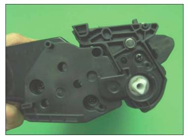
16. Install the P2015 Right End Cap on the right side of the Hopper. Tighten the 2 screws on the Right End Cap.
