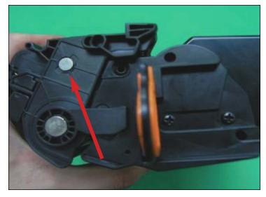
17. Assemble the Hopper side and Waste Hopper together and insert the hinge pin on each side to hold them together.
