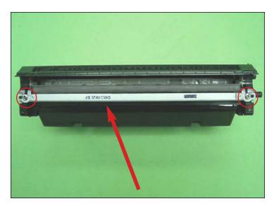
11. Install the doctor blade into the Hopper, and place the Mag Roller wiper on each end of the Doctor Blade. Tighten the two screws (shown) that hold the doctor blade and wipers in place.
