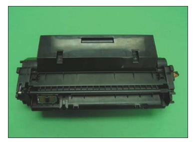
19. Finally, install the Chip, and the conversion from an HP<sup>®</sup> 1320 cartridge to a cartridge that will fit the HP<sup>®</sup> P2015.
