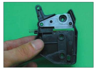
13. Install the Left Stabilizer on the P2015 Left End Cap as shown.
