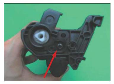
4. Attach the Bearing Plate with screws as shown.
