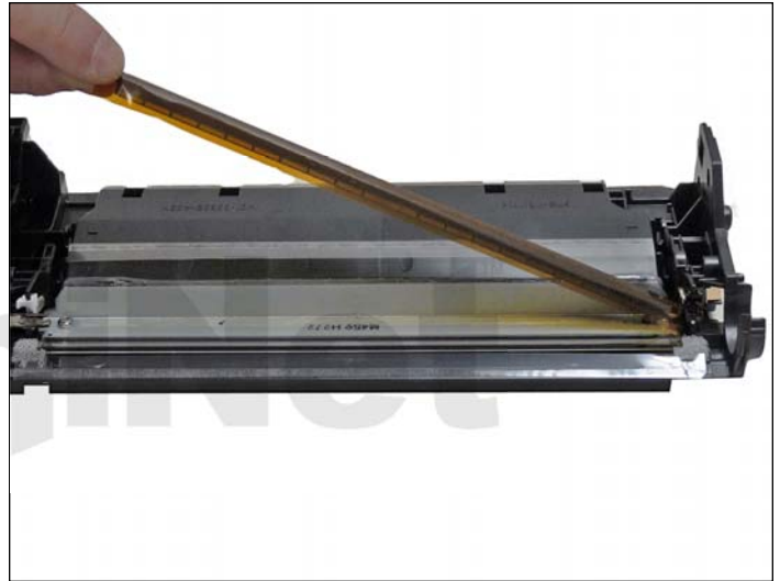
10. To remove the wiper blade, the amber film assembly needs to be removed.
