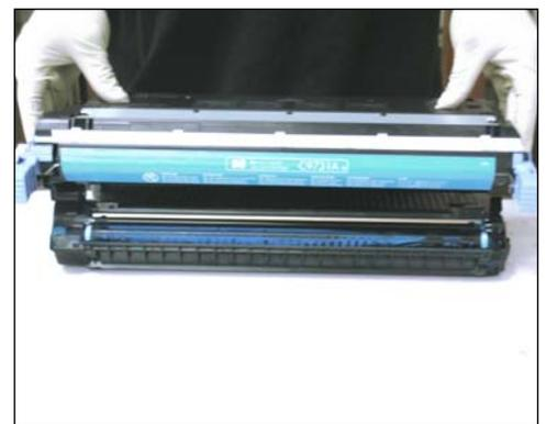
10. Lift and remove the drum unit from the toner hopper.
