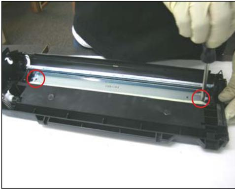
52. Then remove the two screws as shown.
