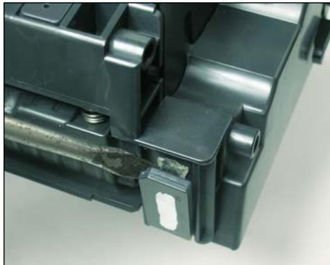
2. Using a small flat head screwdriver, pry the glued chip off as shown.
