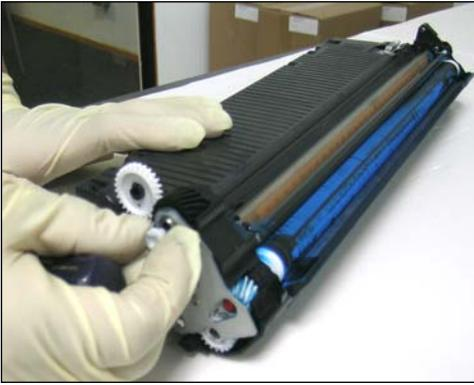
11. Remove the pin bearing as shown.
