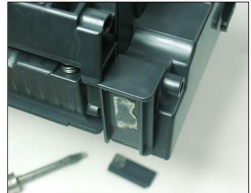
3. Chip removed. It will be replaced later with a new Smartchip.
