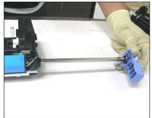
48. Slide the axle out completely as shown.
