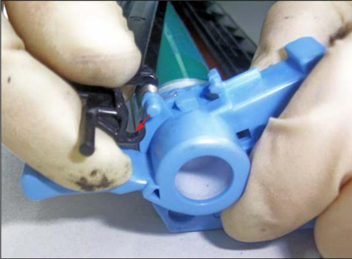
**RELEASING THE DRUM SHUTTER FROM THE DRUM UNIT**
