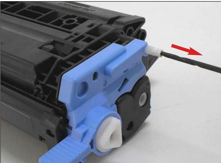
6. Once tool is firmly into the pin, start pulling straight out to dislodge the pin from the cartridge.
