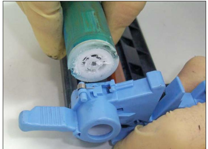
24. Drum shown with spindle severed off.
