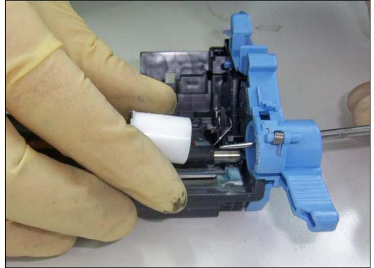
26. Push in the sawed-off spindle out through the end cap as shown.
