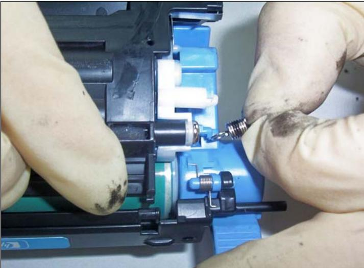
**REMOVING THE TENSION SPRINGS**
