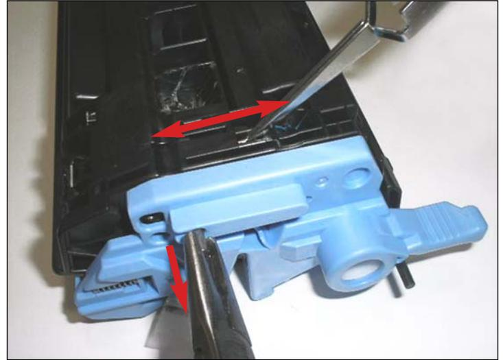
2. Grip the metal pin to pull it out with pliers. using a pair of tweezers, move the top metal tab back and forth while pulling slowly. This will allow disengagement of the pin from the internal contact without breaking the plate. Do not use apply any undue force in pulling. See step 15 explaining the consequences.
