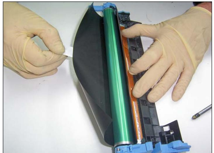
52. The final step in assembling the drum unit is to install the drum shutter. You can choose to unwrap the newly installed drum now and complete this process, or keep the drum covered and continue with the disassembly and cleaning of the developer unit.
