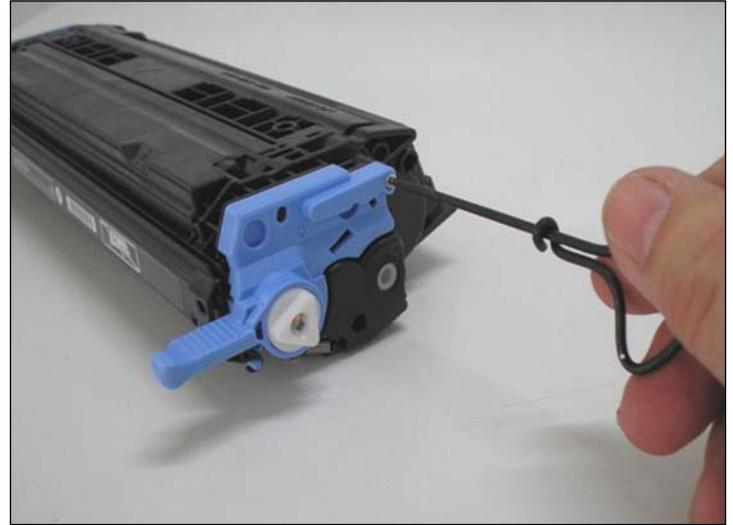
5. Thread the tool 3 or 4 turns into the plastic pin hole.
