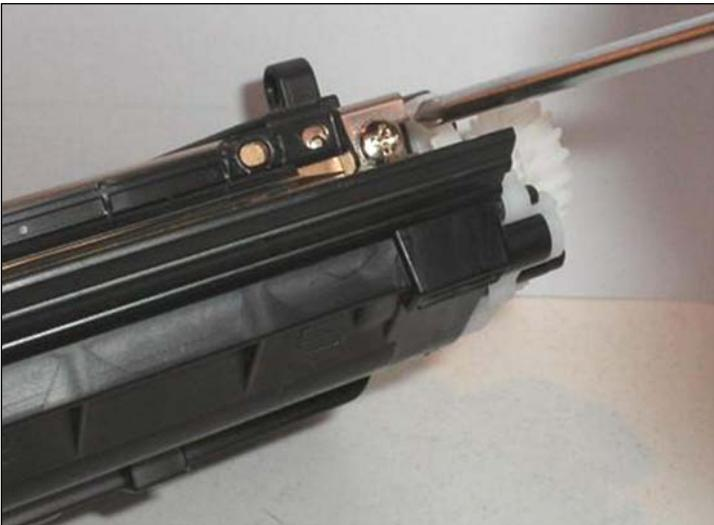
70. Tighten screws at both ends.
