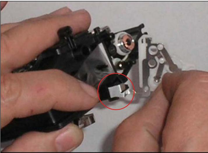
54. Carefully separate the contact plate assembly from the developer unit while keeping the contoured contact (shown) from being distorted, especially at the point of separating it from the pillar.
