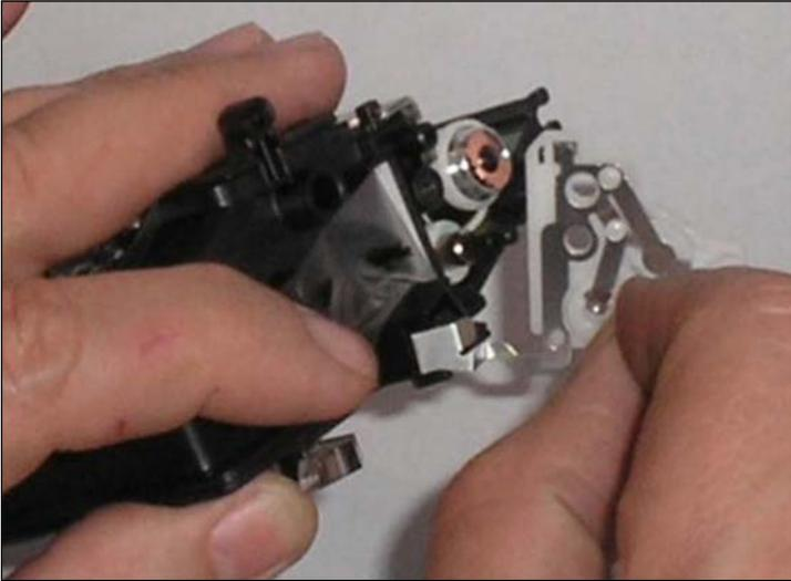
68. Apply a very small amount of conductive grease in the contacts ends, then install the contact plate with the two phillips screws.
