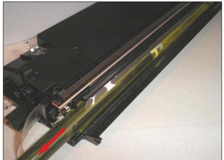
**REMOVING THE DEVELOPER SLEEVE**
