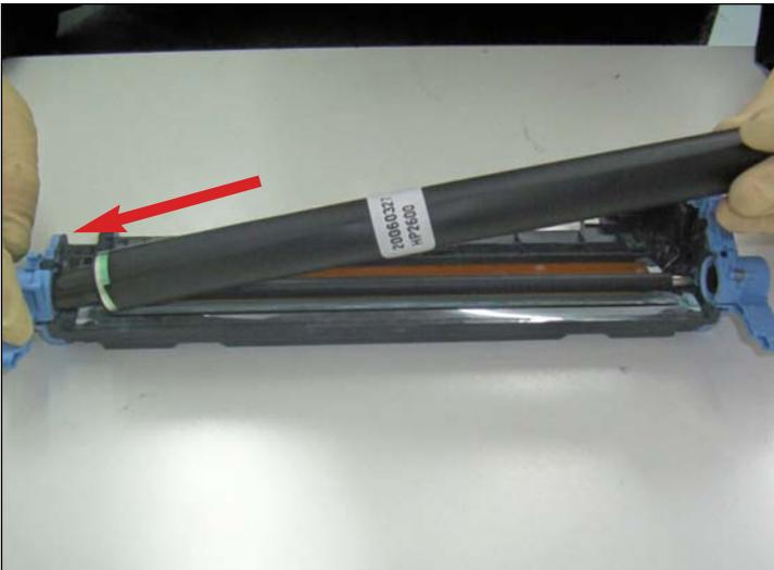
47. Carefully slide the drum with its drive/contact spindle into the axle housing on the left as shown.
