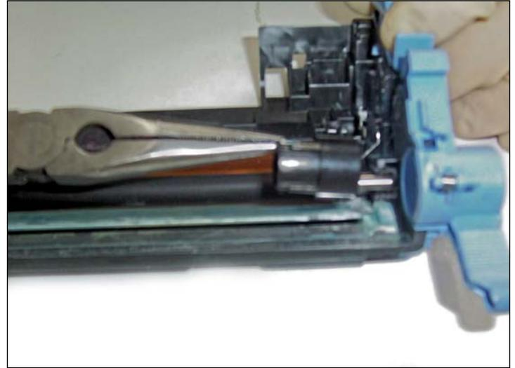
46. First, lubricate the blue axle housings with a minimum amount of white bearing grease.
