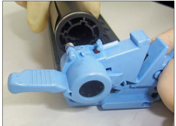
48. Lower the opposite end of the drum into place as shown. Align flange with the axle attachment.
