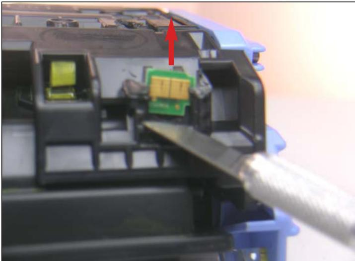
77. Slide the blade beneath the base of chip and begin lifting it up carefully, sliding it out through the slotted housing as shown.
