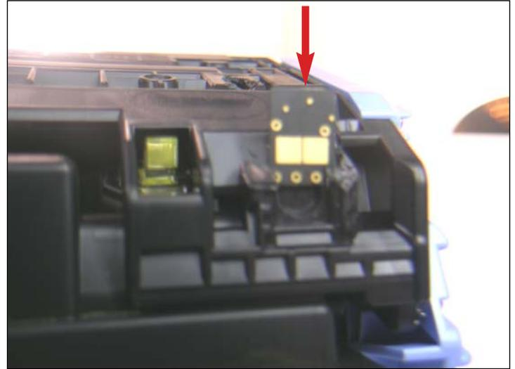
80. Insert the new chip into the slots with the golden contact position shown.
