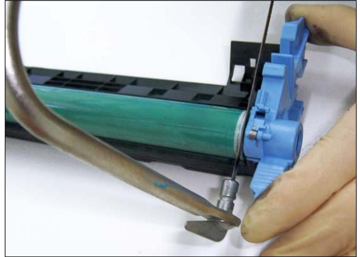
22. Rotate drum 90° counter-clockwise midway the cut to avoid going too deep and damage components.
