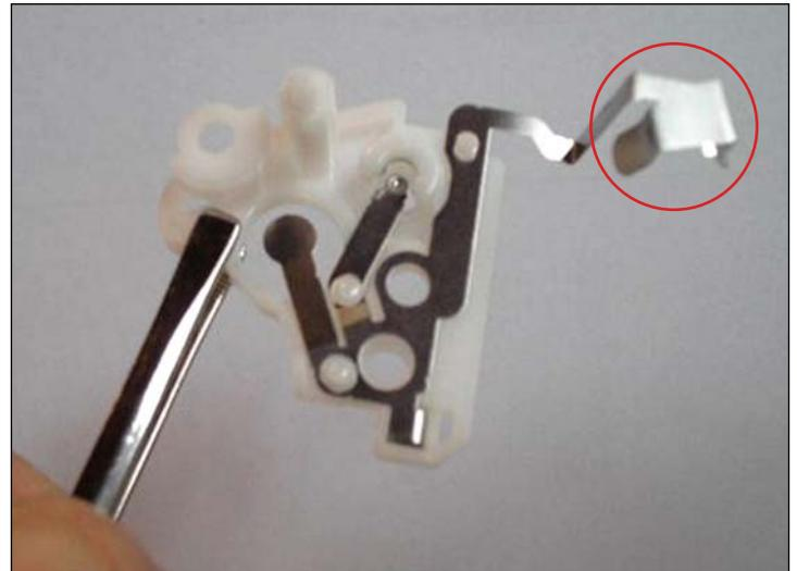
55. Contact plate removed with contoured contact shown intact.
