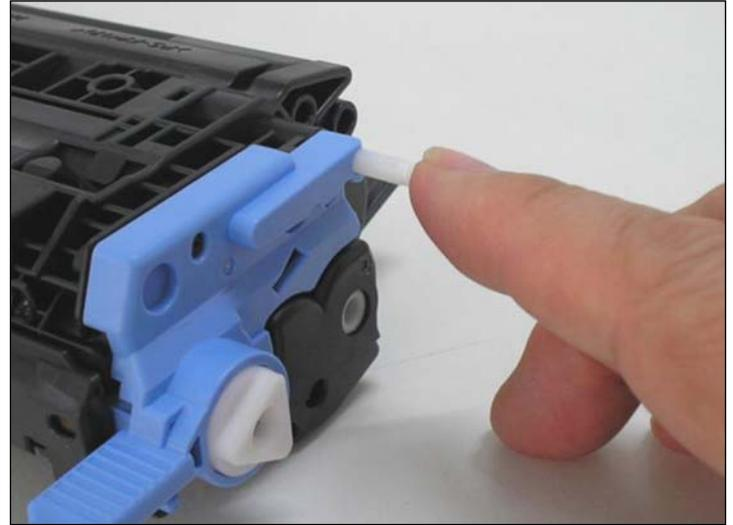
72. Insert the plastic pin by hand mid way.
