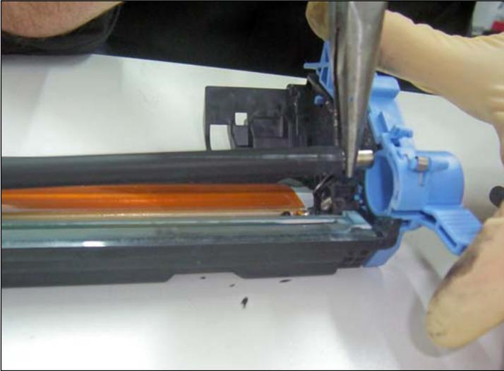
**REMOVING & CLEANING THE PCR**
