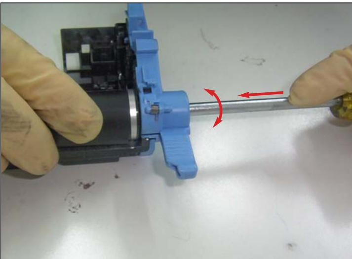
51. Rotate the spindle back and forth to align it with the OPC.
