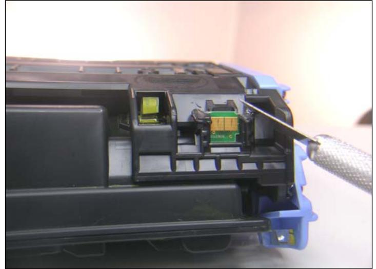
76. Using an X-Acto knife, carefully cut away the melted plastic tabs above the chip that anchor it into place.
