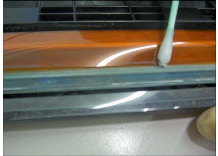
40. Using a cotton tip swab, clean the edges and underlining of the PCR blade.
