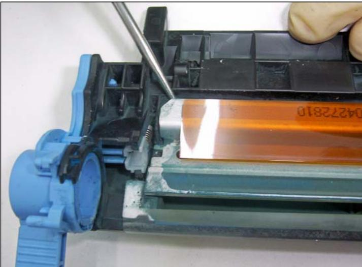
33. Use a scribe or flathead screwdriver to pry the wiper blade assembly from its adhesive seal.
