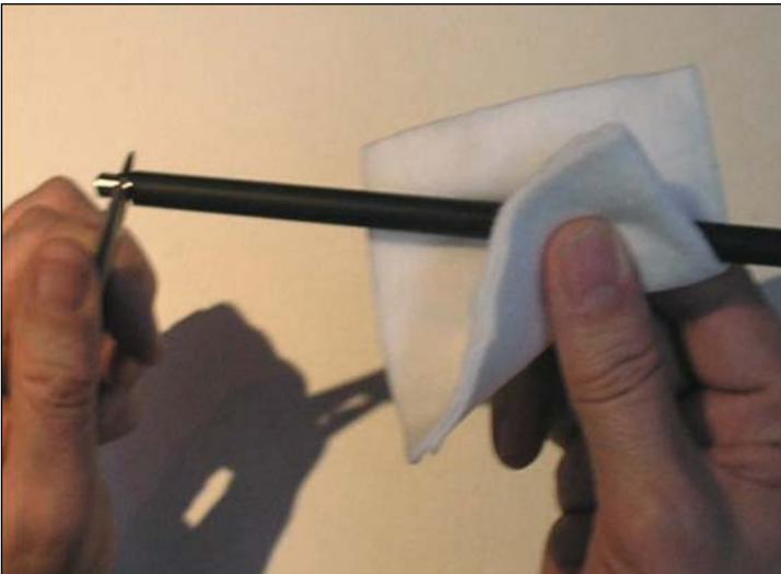
30. Clean with a small amount of water and mild soap in case of contamination, otherwise use a simple dry pad.
