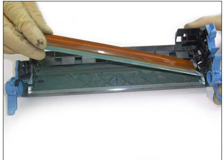
34. Lift the wiper blade out from one side and to the next.
