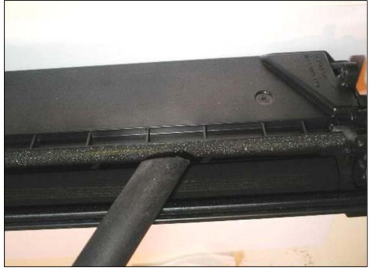
65. Vacuum the toner from the roller and from the hopper. Secure foam seal at each end.
