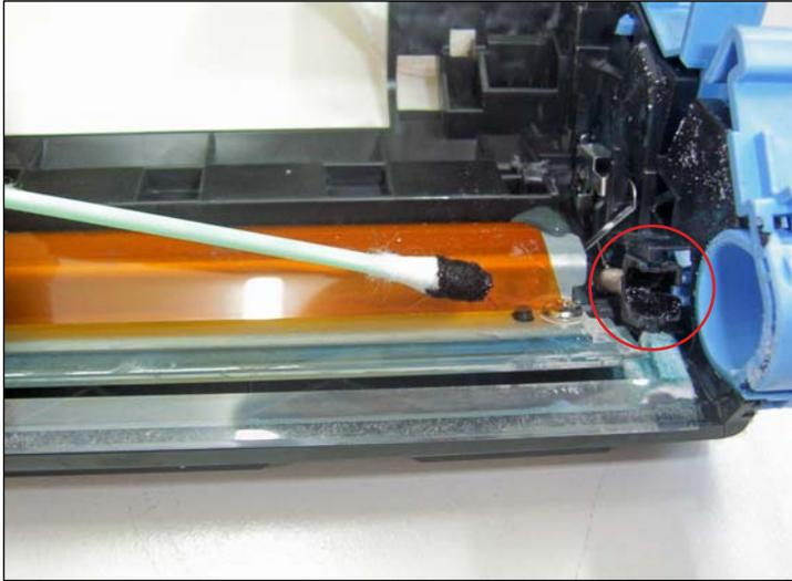
43. Apply a small amount of conductive grease onto the black PCR saddles on both sides. Do not over-lubricate.
