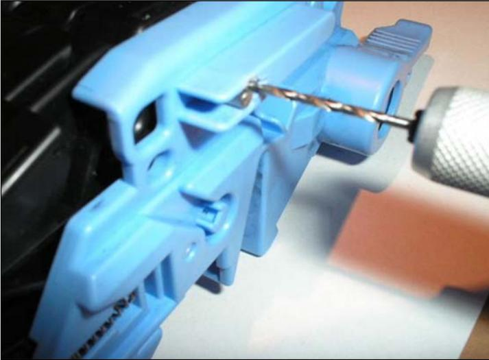
**CARTRIDGE DISASSEMBLY: METAL PIN REMOVAL**
