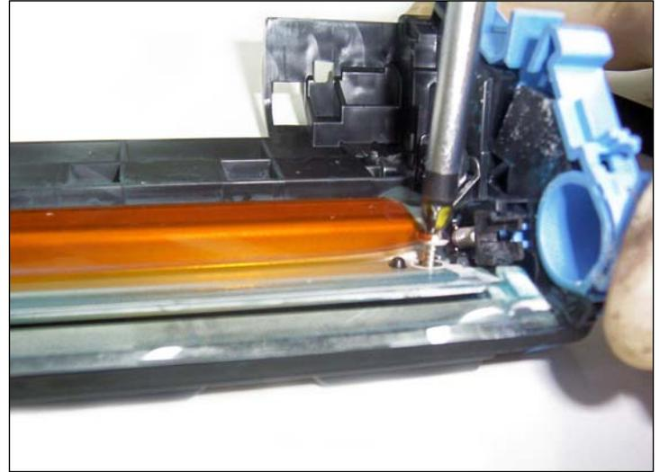
32. Be careful not to crease or damage the PCR contact strip attached.
