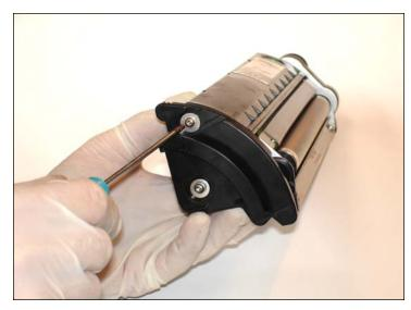
4. Remove the two torx security screws from the colour cover side using a Security torx screwdriver.
