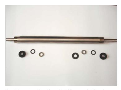
24. DVR washers & bushings should be assembled as shown.
