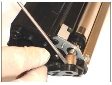
18. On the other part, remove the metal develop endplate which fixes the develop base.
