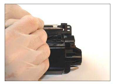
8. Push carefully the black end cap tap as shown using a straight hook tool.
