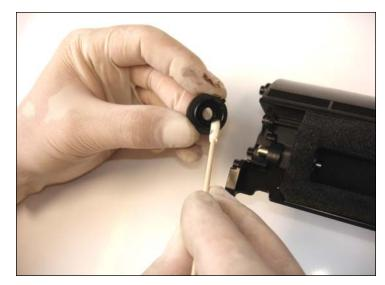
28. Clean the black add roller bearings with a cotton tip swap with isopropyl alcohol.
