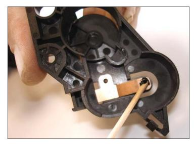
36. Clean the residual toner of the electrical contact with a cotton tip swap with alcohol isopropyl. Apply conductive grease to lubricate it. Place the end cap in the gearless side with the screw and the tab.
