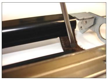
26. Comb both side foams with a flathead screwdriver to prevent leaking. Insure the good conditions of the foam and black mylars. Otherwise it can cause massive leaking. In case of toner adherence in the toner mylar surface, use a cotton tip swap gently to eliminate all residual toner.
