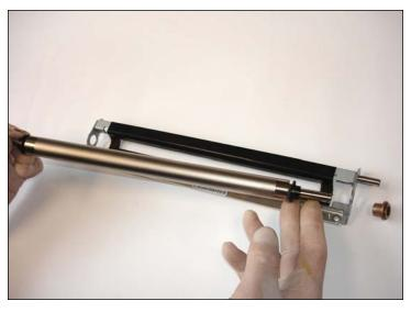
30. Place the develop roller and reassemble its parts in reverse order.
