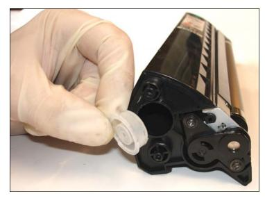
16. Remove the toner fill cap from the gearless hopper side and clean out any remaining toner.
