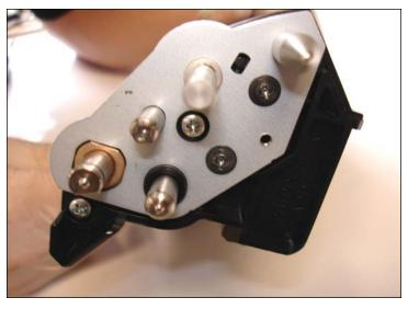
34. Place the metal gear support endplate until it fits properly with the previous installed bearing.
