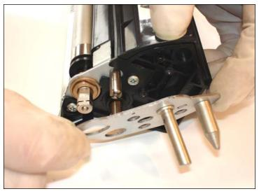
14. Release the metal gear endplate.
