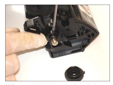
20. Remove the black add roller bearings from both sides.
