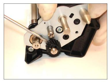
12. Carefully pull out the shaft using a flathead screwdriver between the black gear and the metal gear plate.
