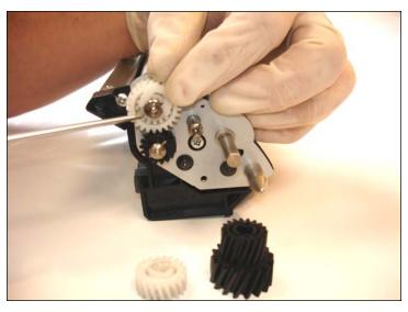
10. After releasing the two unblocked gears carefully, remove the white plastic "U"-shape clip from the DVR guide gear.
