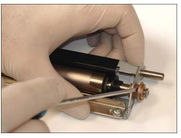
22. Release the fixing bearings of the develop frame.
