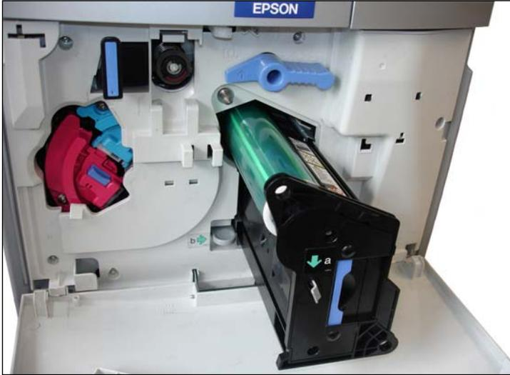
1. Release the drum unit turning the blue drum unit blocker lever one quarter counter clockwise.
