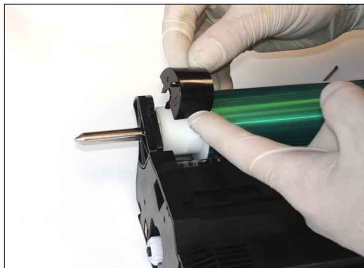
12. On the other side of the drum, remove the plastic black drum gear cover.
