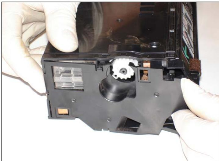
47. Place the gear end plate by left side to preserve the tabs.
