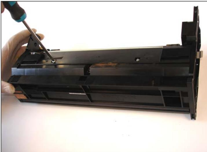
19. Remove the two screws on the bottom black cover of the cartridge.
