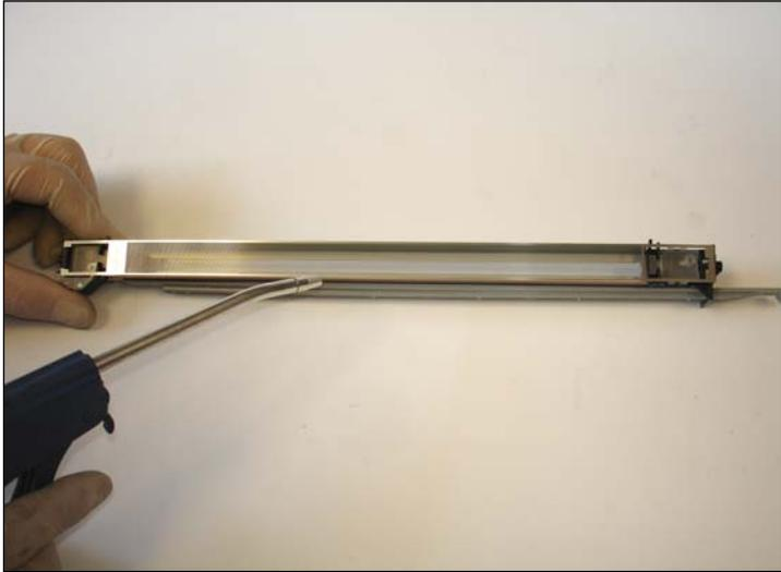
41. Before installing the corona, clean it with air compressed as shown.
