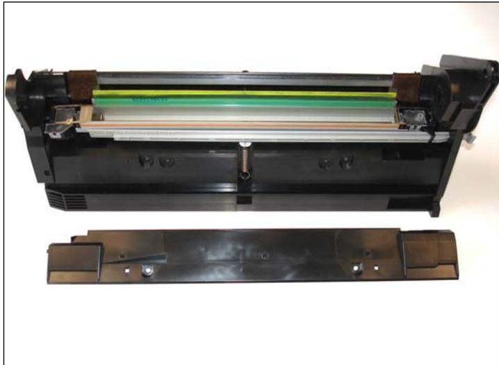
45. Cartridge view with its bottom cover uninstalled.
