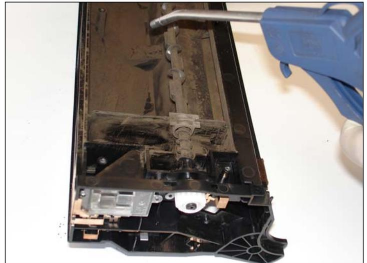
32. Clean the waste hopper with compressed air.
