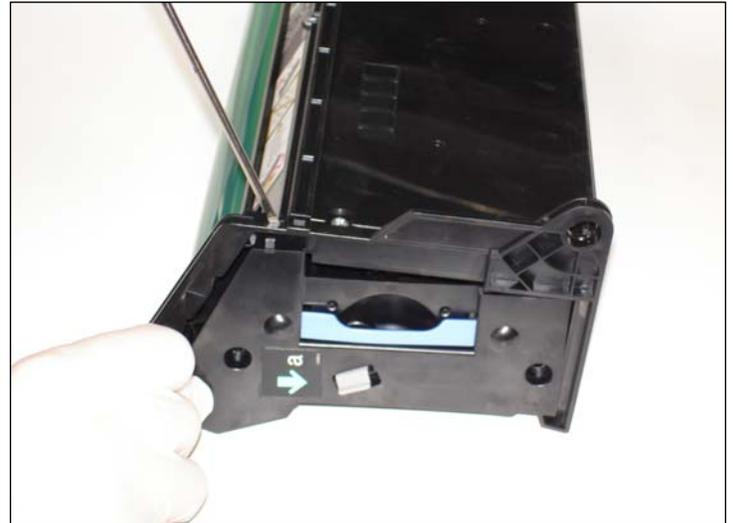
8. Release the black end cap using a small flat head screwdriver to press the tab as shown.
