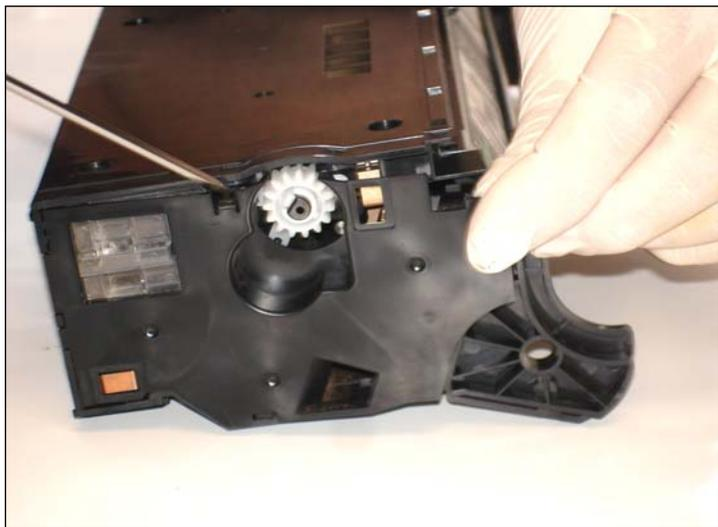
15. Release the gear end plate tab on the other side of the cartridge using a hook tool.
