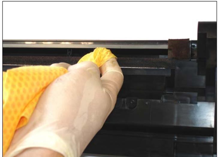
36. Clean the recovery blade with a cotton tip swap or a toner grabber with alcohol isopropyl mixed with distillate water. Be careful to don't damage or bend the blade since it would cause spotting.
