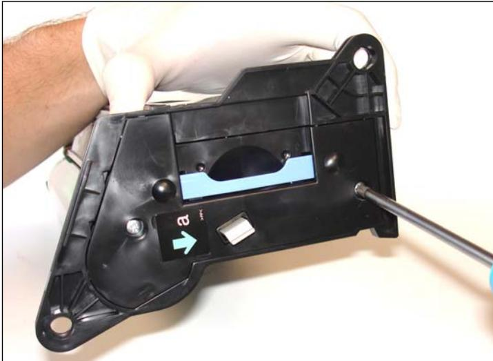
7. Remove the two Phillips screws from the black handle end cover.
