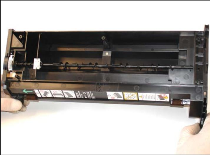
33. General view once cleaned. Clean as best as possible the plastic yield sensor window placed in the waste toner section to avoid a “full waste toner” message on printer’s display.
