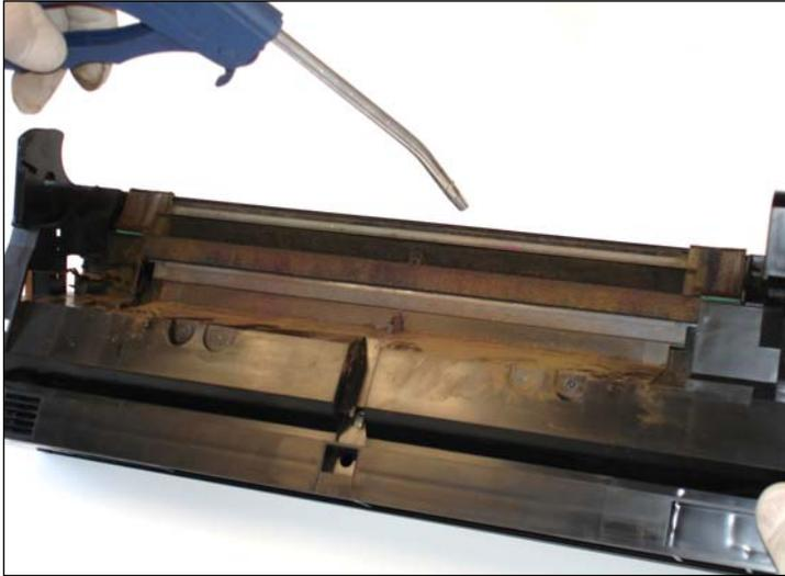
29. Blow the hopper with compressed air to clean out any remaining waste toner.
