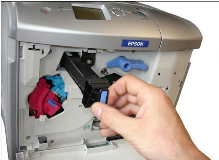
3. Check and Clean if necessary the ozone filter with compressed air. Keep it horizontal and don't shake it before cleaning.
