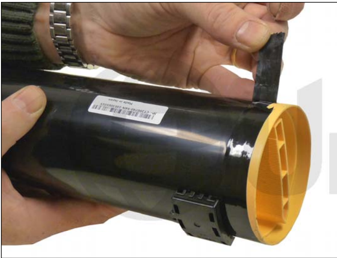
1. Remove the tape from the colored end cap.
