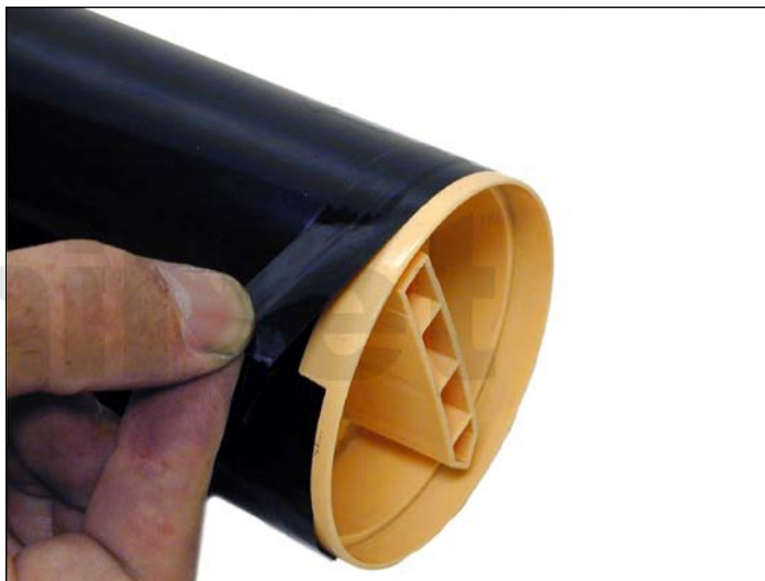
4. Replace the end cap, replace the tape.
