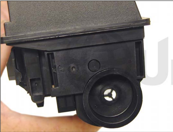
3. Re-install the fill plug.
