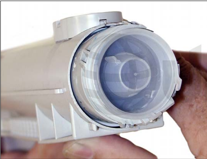
5. Replace the fill plug and end cap.
