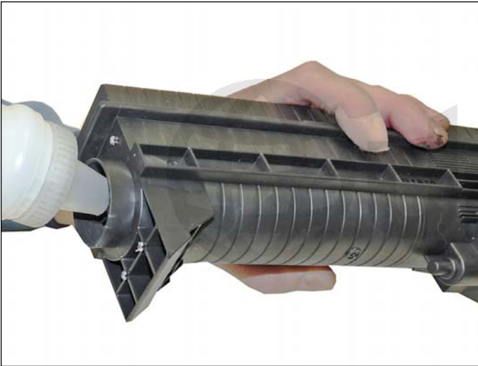
6. Fill the hopper with new toner for Canon C3200 and replace the fill plug.
