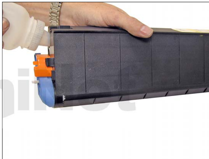
2. Make sure the toner port is closed before refilling.
