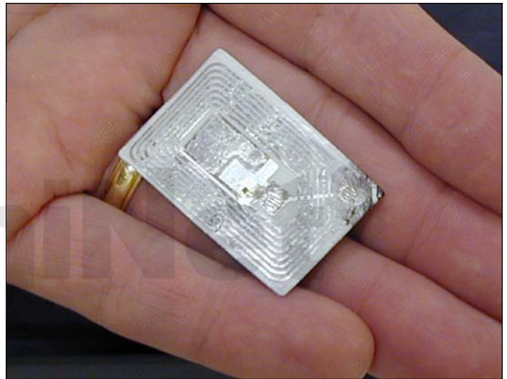
5. Replace the RF type chip (the chip is manufactured into the label).
