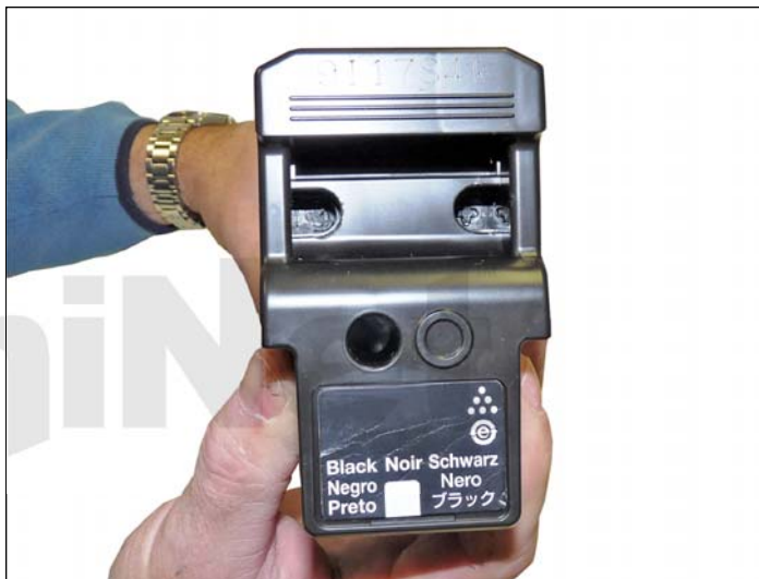
7. Install the end cap on the cartridge. An easy way to do this is to place four drops of hot glue on the four broken posts. Quickly place the end cap on before the glue dries. If further help is necessary to keep the end cap on, black tape along the seam works well.
