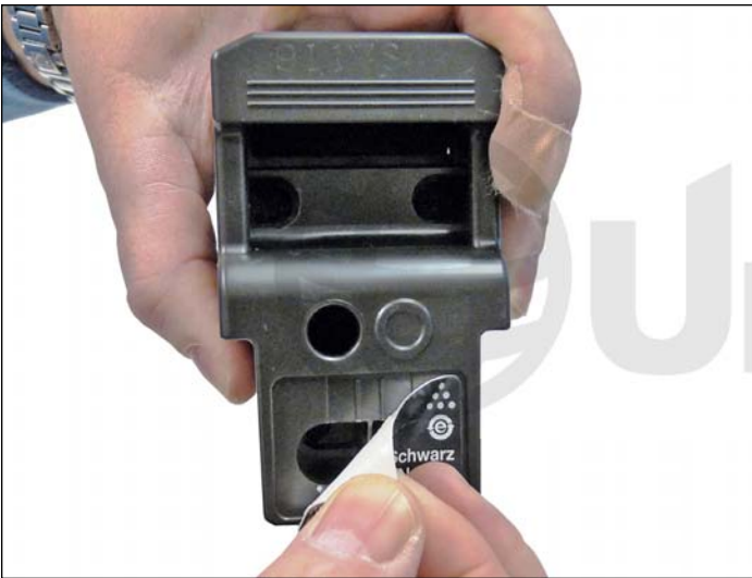
2. Remove the Cartridge ID label from the end cap.
