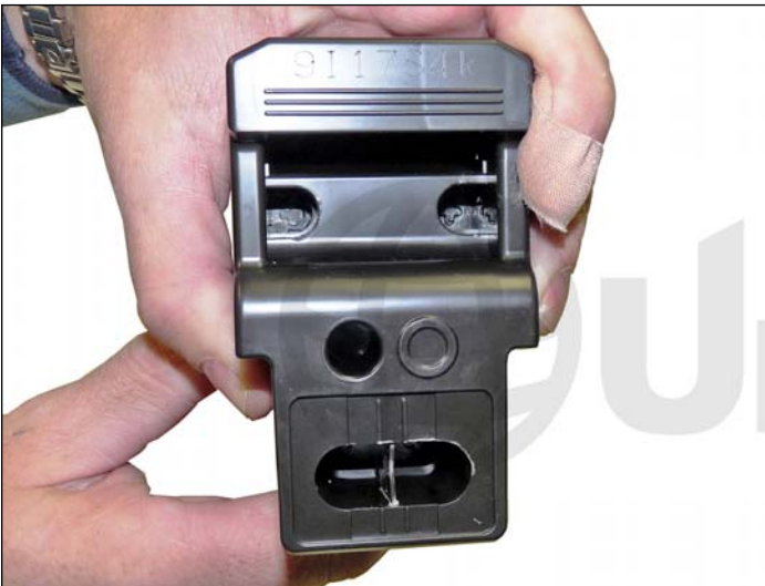
3. Remove the two remaining welds in the same manner as Step 1.
