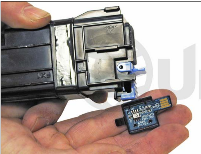
9. Slide the holder out of the cartridge and replace the chip.
