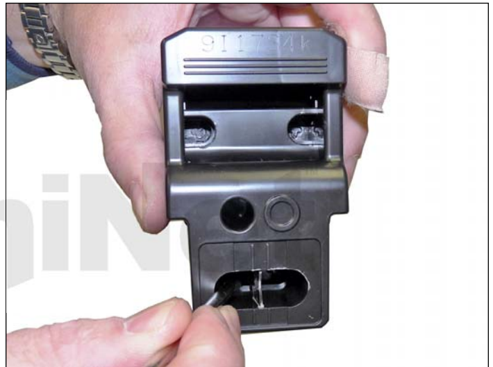
3. Remove the two remaining welds in the same manner as Step 1.
