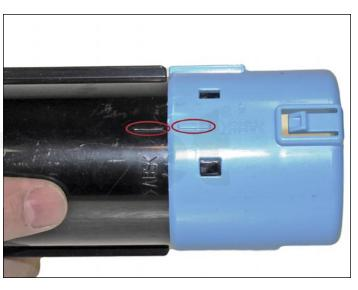
6. Align the two marks on the end cap and tube.
