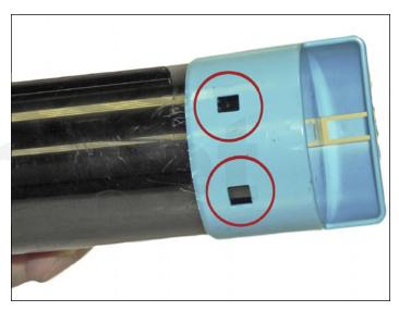
1. Pry up on the colored end cap by lifting up all four tabs.
