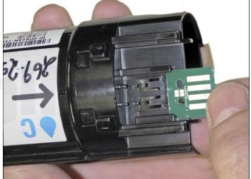
7. Using a small Jeweler's type screwdriver, pry up the chip through the small slots underneath and slide it out.
