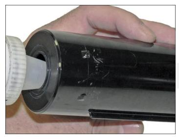
5. Fill the cartridge with toner for use in the Dell 5130. Replace the fill hole seal (as shown). If the seal is damaged or is leaking the seal for the Samsung CLP-300 can be used.
