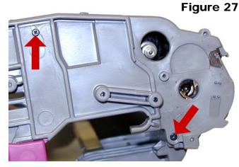
25) On the opposite side, remove the two small Phillips head screws from the frame as indicated. See Fig.  $\bf 28$
