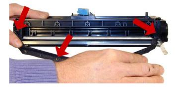
10) Clean the Doctor Blade with a cotton swab and a small amount of acetone. Remove any remaining residue with another cotton swab and 99% Isopropyl alcohol.
