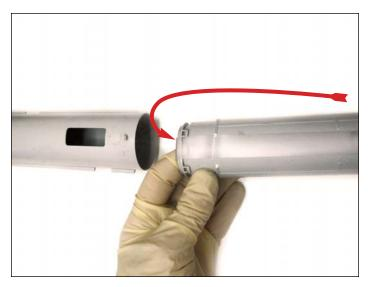
14. gently wrap the seal flap around the toner fill opening (as shown) while you prepare to insert the cartridge. This will ensure that the seal flap properly exits the opposite end of the container.
