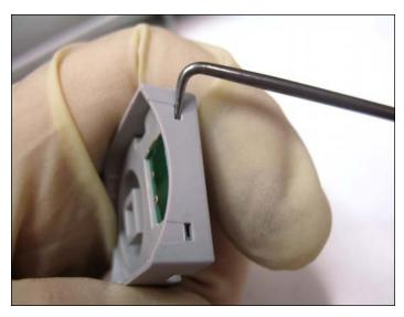
25. Unlock the actual chip from its housing by pressing the tabs (shown) using an angled hook tool.
