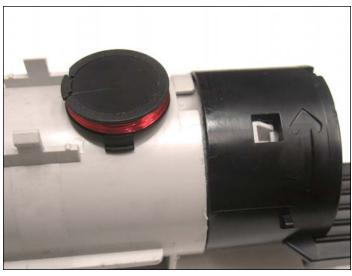
**INSTALLING THE NEW CHIP**27. Place the new contact chip on the cartridge in the manner shown.
