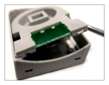
26. Carefully lift the chip from its housing.
