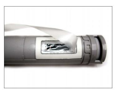
13. Remove the adhesive backing of the **Clearseal**™ and carefully place over the opening as shown. Apply pressure using your fingers to ensure a tight seal.
