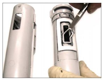
**ALTERNATE CLEARSEAL™ ASSEMBLY**10. First, using a pair of pliers, gently peel off the worn sealant (shown) from the toner cartridge.
