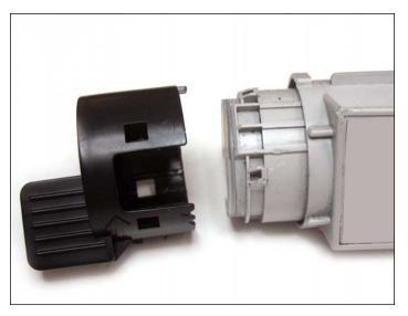
4. Carefully slide out the gearless end cap. **NOTE**: Note the original positioning (shown) for reassembly.
