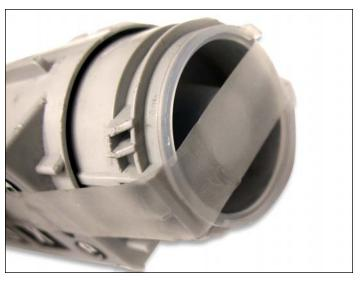
19. First, wrap the remaining seal around the toner fill plug as shown.
