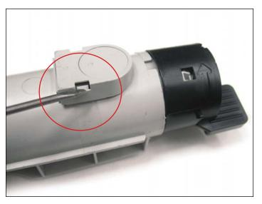
23. Using a small flathead screwdriver, press down on the tabs (shown on either side) to release the chip housing.
