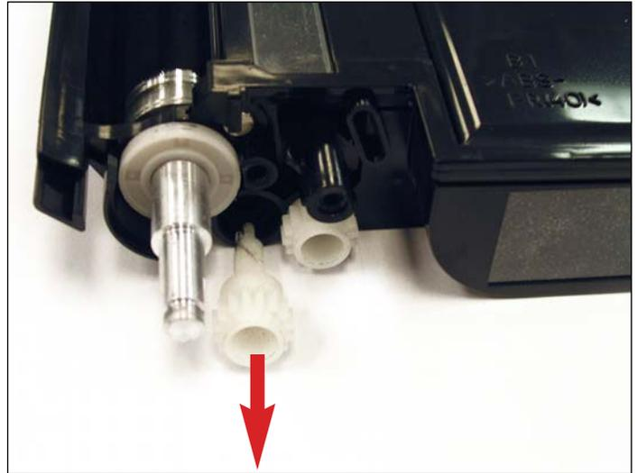
11. Remove the front auger drive gear as shown. This will allow you to remove the bearing.
