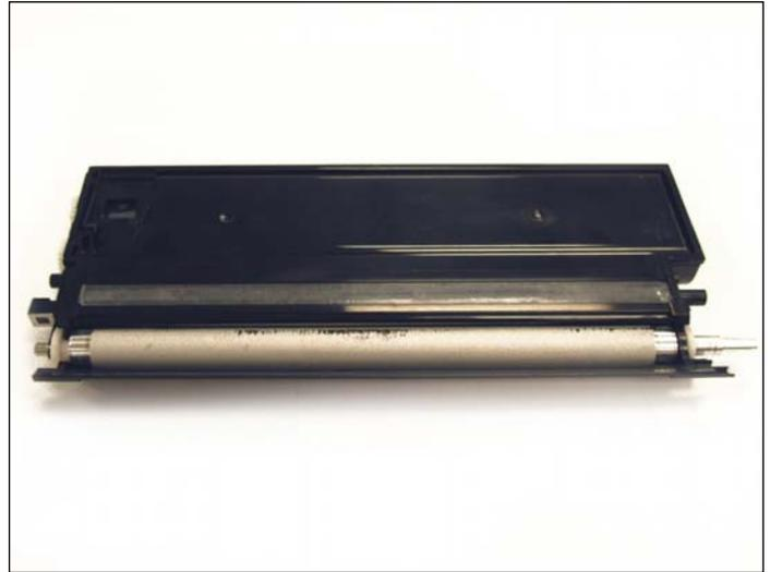
22. Once you have filled the carrier, clean the edge with isopropyl alcohol and install a new carrier chamber seal.
