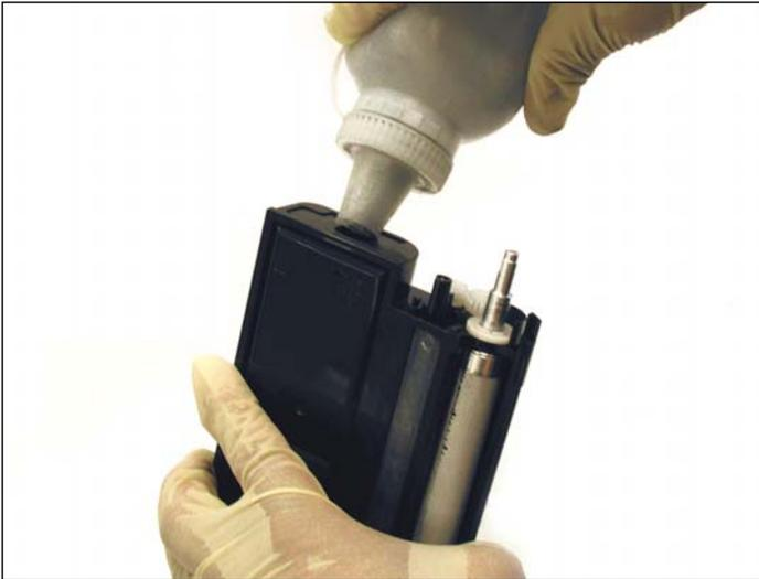
23. If a standard cartridge is being used, this will be a good time to fill the cartridge. Seal the cartridge using the OEM sealing strip or an aftermarket sealing strip.
