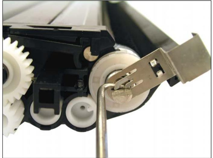
9. Continue by sliding the contact off using a small hook tool. To do so, position the hook tool between the contact (as shown) and pull off.
