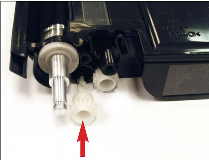
19. Once the bearings are installed position the front auger drive gear as shown.
