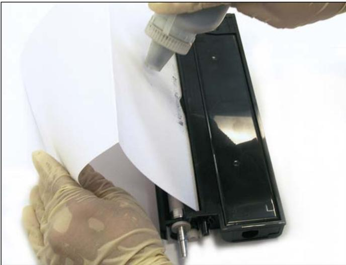
21. Using a piece of paper (size is your choice) position it inside the carrier chamber blocking the Mag roller. This will simplify filling the carrier chamber.
