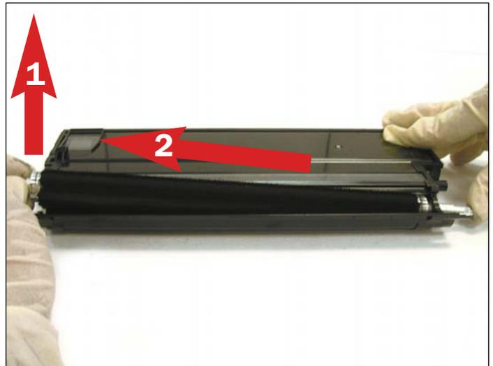
15. Remove the Mag (as shown) and clean using compressed air to blow off all the remaining toner.
