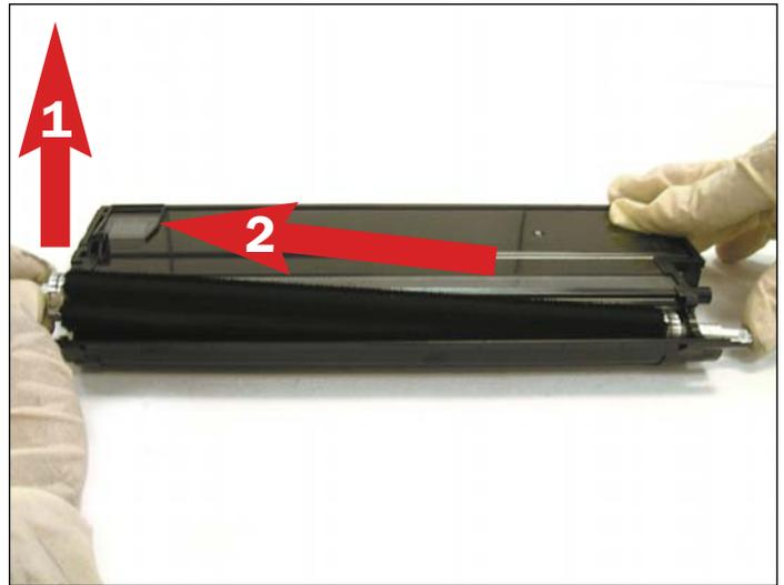
13. The fastest way to remove the support bearing on the opposite side is to first lift the Mag roller. Pull it out about 5 mm, then stop and position the Mag roller back in the cartridge.
