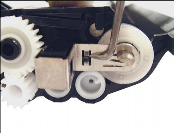
8. Remove the Mag Roller contact by first releasing it from the tab as shown.
