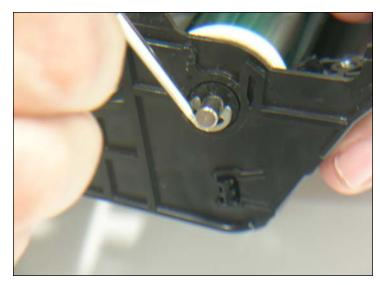
18. Remove the shaft of the drum by releasing the retaining washer from the left side of the cartridge.
