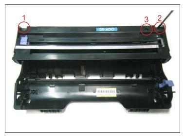
12. With a medium size Phillips screwdriver remove the screws securing the corona wire assembly. There are two in each corner holding the plastic top and one, visible thru the hole on the right hand side securing the electric contact of the control grid and the cleaning felt.
