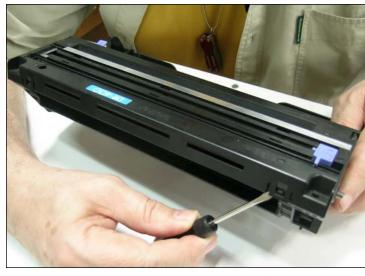
29. Insert the lid containing the corona assembly, align the four clips, and press down to clamp it.
