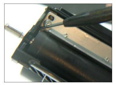
3. On the same side and with the help of a small jeweler screwdriver release the three (3) clips holding the developer roller bearing cap to the toner hopper. The first clip is right below the screw holding the developer blade, the opposite clip is between the side of the roll and the casing while the third one is accessible from outside the casing.
