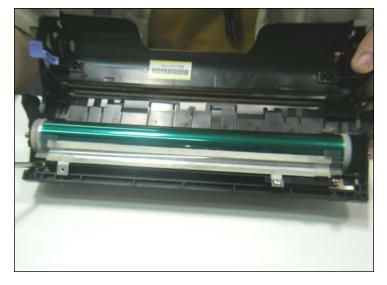
27. Insert the drum cleaning assembly and with a Phillips screwdriver and tighten the screws to secure it to the cartridge. The screw on the left will pressure the contact between the assembly and the drum axle.
