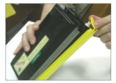
11. Insert the OEM or the compatible yellow seal cover for the developer roller to protect it during transit.
