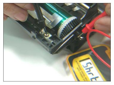
28. With a Tester check the electrical continuity between the contact of the assembly and the drum shaft.
