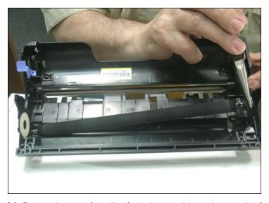
24. Extract the transfer roller from the cartridge using a pair of long nose pliers. Notice that the saddles and the helical gear will also come out. Clean the roller with compressed air or vacuum cleaner. DO NOT USE any solvent or chemicals on the transference roller.
