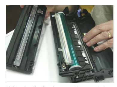
14. Clean the grid surface of any toner with compressed air.
