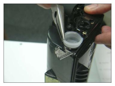
8. Remove the fill plug from the hopper. Discharge any toner from the toner hopper. Use dry compressed air or a vacuum to THOROUGHLY clean out the toner hopper. Clean the developer blade using a dry lint free cloth.
