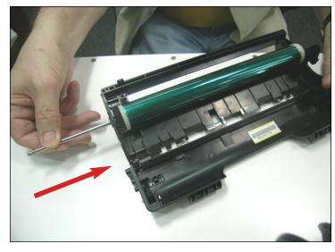
26. Slide the axle from left to right, insert the bearing in place and the retaining washer to secure the axle in place.
