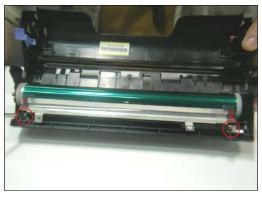
16. With a Phillips screwdriver remove the screws holding the drum cleaning assembly. You will notice that it is composed of a cleaning felt, a recovery blade and a couple of scraper-blades.
