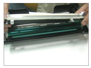
17. Remove and clean the assembly thoroughly removing all remains of old toner.
