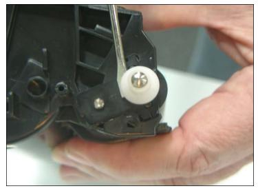
1. With the use of small flat blade screwdriver, slightly pry up the white plastic alignment hub located from the non-gear side of the developer roller and remove it.
