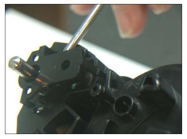
4. With a small flat blade screwdriver, pry the bearing cap off the developer roller axle and the fixing post.
