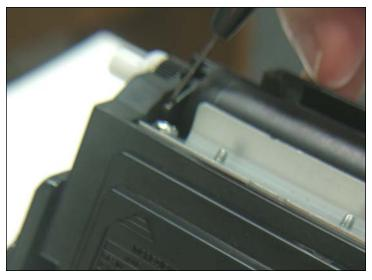
5. Move to the other side of the cartridge and above the white plastic hub on the gear side, locate the clip that holds the developer roller cap-bearing. NOTE: Contrary to the other bearing cap this one is located between the developer roller and the side of the cartridge.
