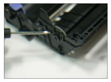
23. NOTE: There is also a plastic stabilizer bearing for the axle located on the same side of the clutch gear which must be secured.
