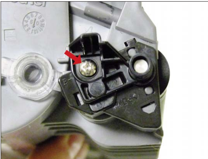
17. On the non-gear side, install the outer axle plate cover and screw.
