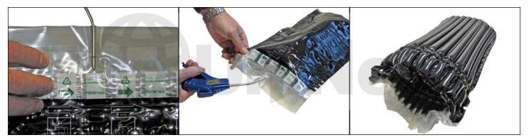
1. Inflate the bag by inserting the air gun nozzle into the center fill port of the bag as shown
