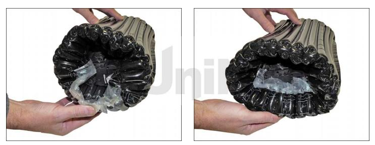
3. Hold the outer edge of the bag into the center of the bag to lock the cartridge in place.
